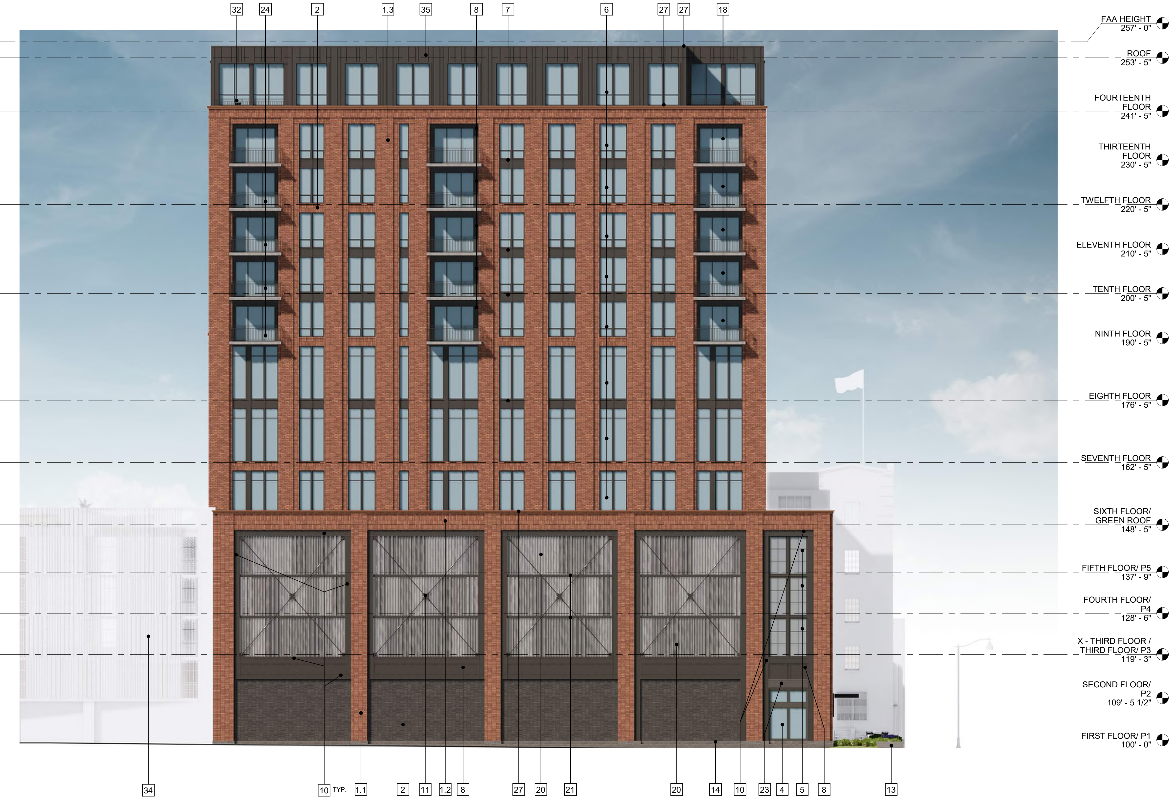
1 EAST BUILDING ELEVATION 3/32" = 1'-0"
