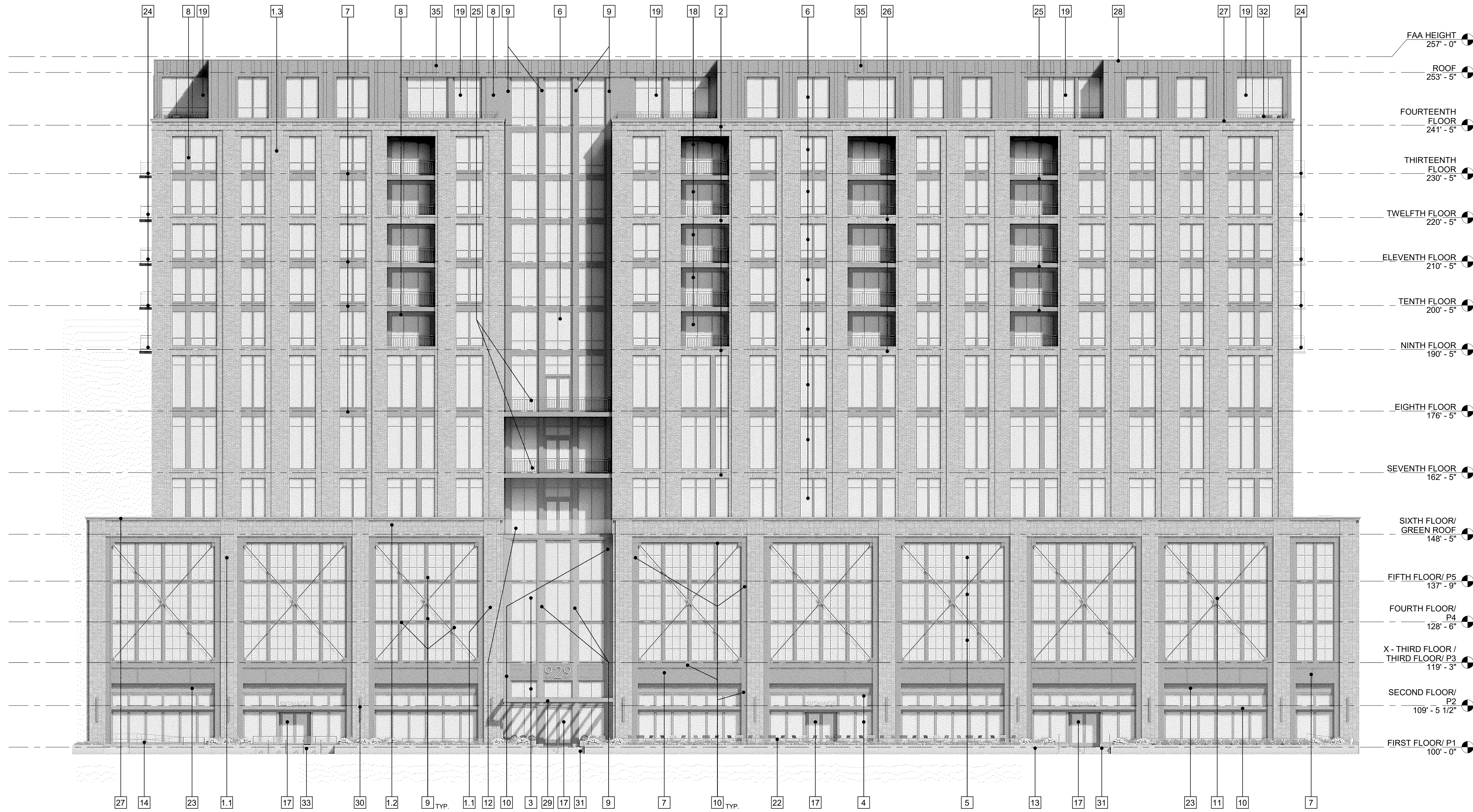
1 A221 NORTH BUILDING ELEVATION - EAST WASHINGTON AVENUE 3/32" = 1'-0"
