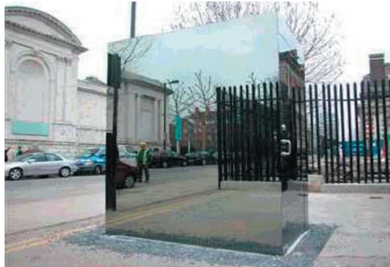
A London artist-designed public toilet built with one-way mirrors: users inside can see outside, but passersby only see a reflection of themselves.
