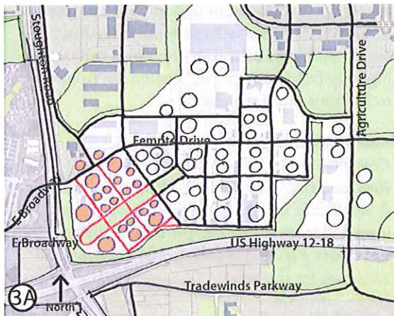
Gateway Area Phasing Plans: Phase 1 includes new streets (red) and development opportunities (salmon) focused primarily in the northeast part of the area (1), Phase 2 makes additional connections and buildings extending toward the southwest and the U.S. Highway 12-18 and Stoughton Road intersection (2), Phase 3A shows build-out without flyover (3A), and Phase 3B shows build-out with flyover (3B).
