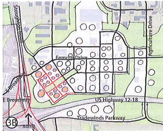
Gateway Area Phasing Plans: Phase 1 includes new streets (red) and development opportunities (salmon) focused primarily in the northeast part of the area (1), Phase 2 makes additional connections and buildings extending toward the southwest and the U.S. Highway 12-18 and Stoughton Road intersection (2), Phase 3A shows build-out without flyover (3A), and Phase 3B shows build-out with flyover (3B).
