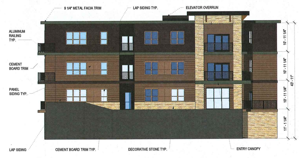
3 SOUTH EXTERIOR ELEVATION 3/32" = 1'-0"
