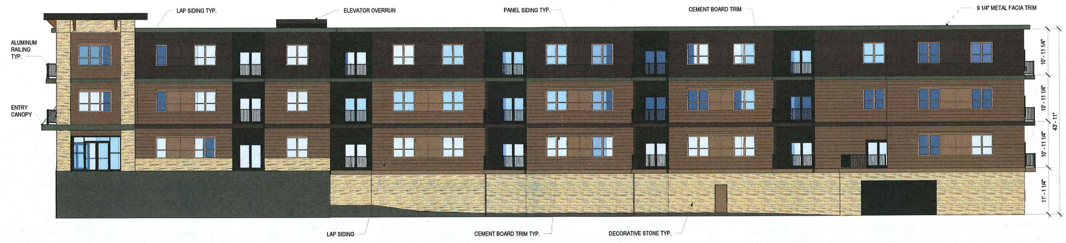
1 EAST EXTERIOR ELEVATION 3/32" = 1'-0"
