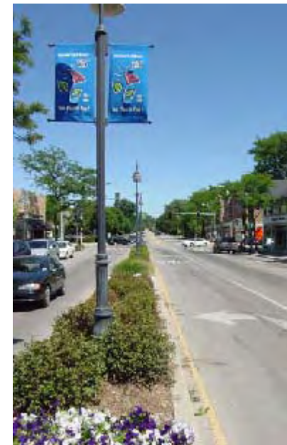
Figure I-3: Traffic Calming: Landscaped Portion of a Pedestrian Refuge Median in Downtown Glenview, Illinois
