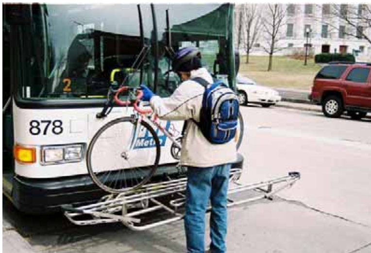
Bike Rack on Madison Metro Bus. Image: Della Haugen, Bicycle Federation of Wisconsin
