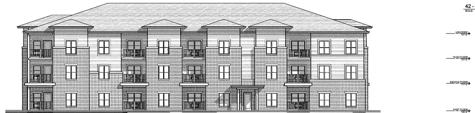
42 - UNIT NORTH ELEVATION SCALE: 1/8" = 1'-0"
