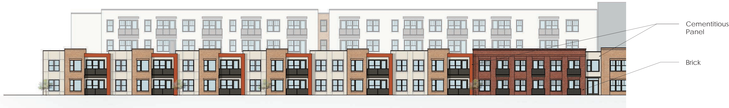
2 East Main St. Enlarged Elevation Scale: 1/32" = 1'-0"
