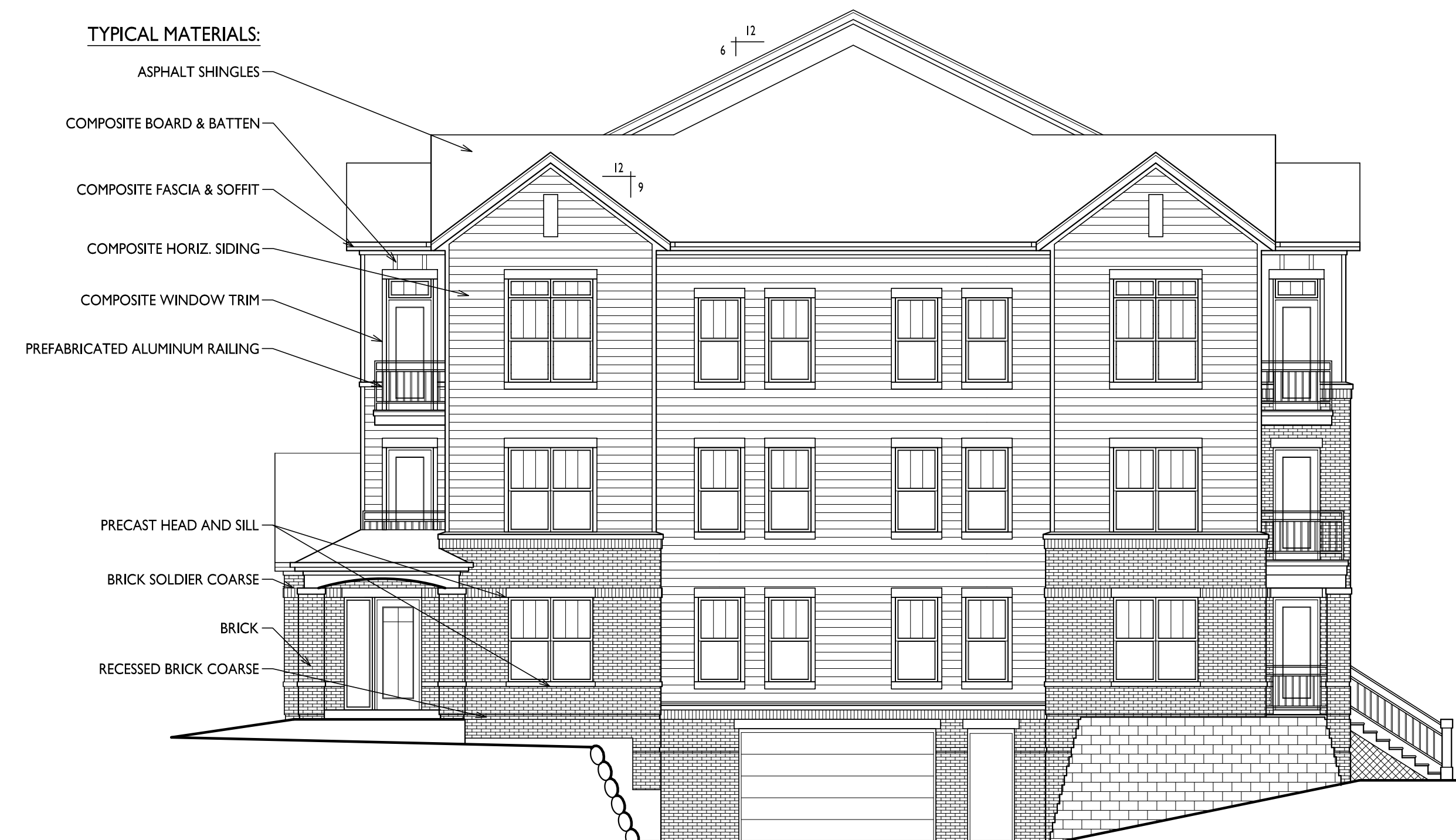
BUILDING #1 SOUTH ELEVATION 2 A-2.2 1/8"=1'-0"
