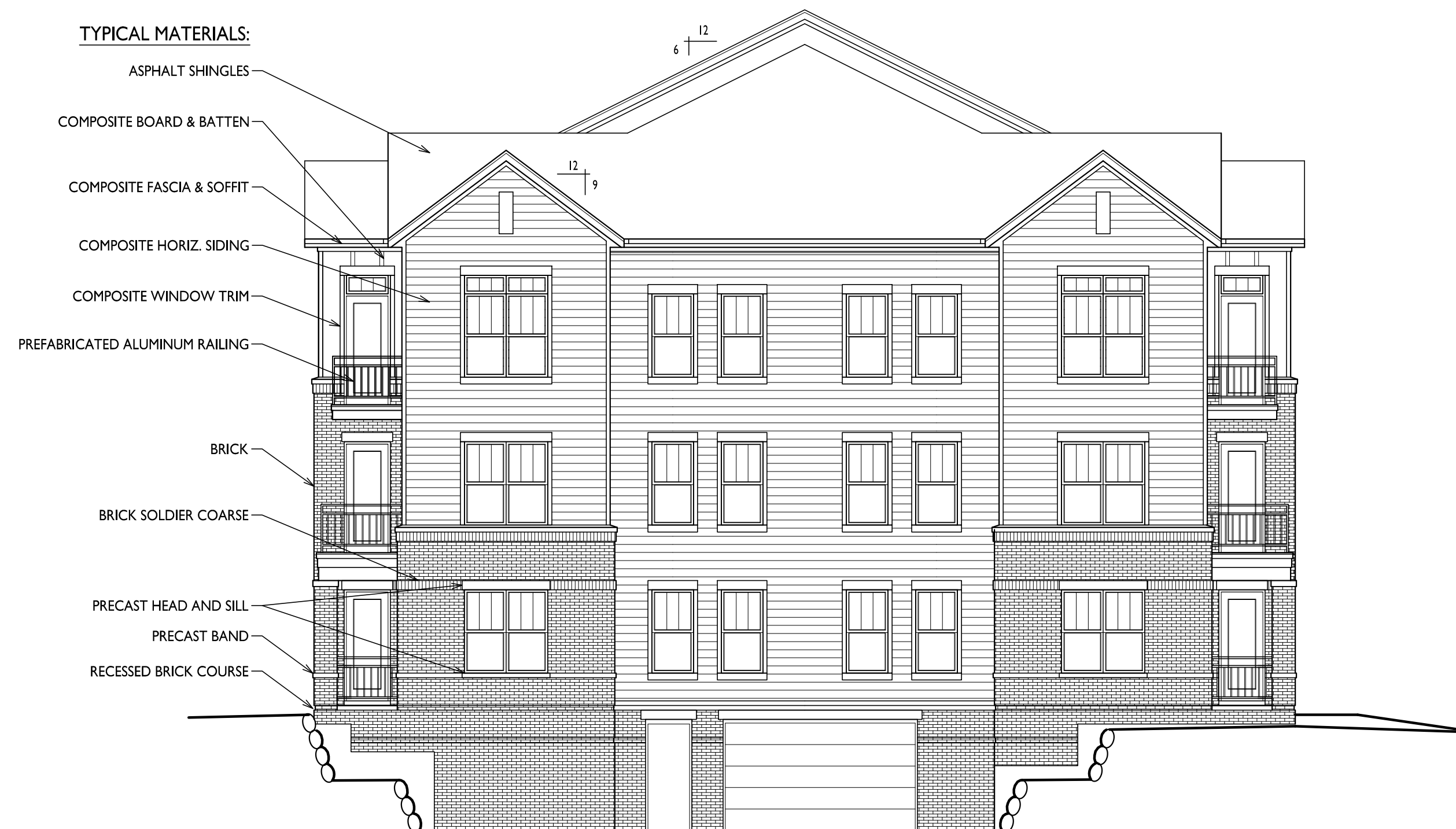
BUILDING #2 SOUTH ELEVATION 2 A-2.2 1/8"=1'-0"
