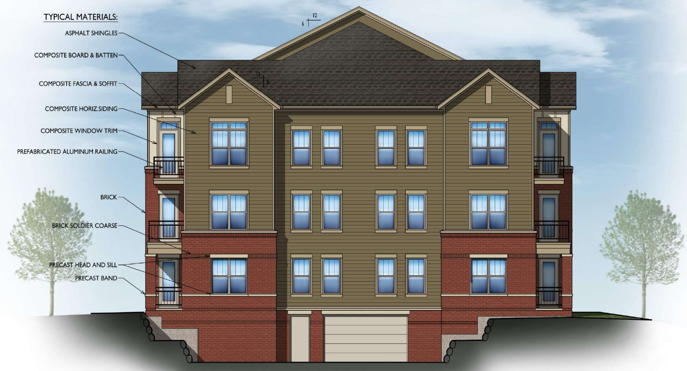
BUILDING #2 SOUTH ELEVATION 2 A-2.2 1/8"=1'-0"
