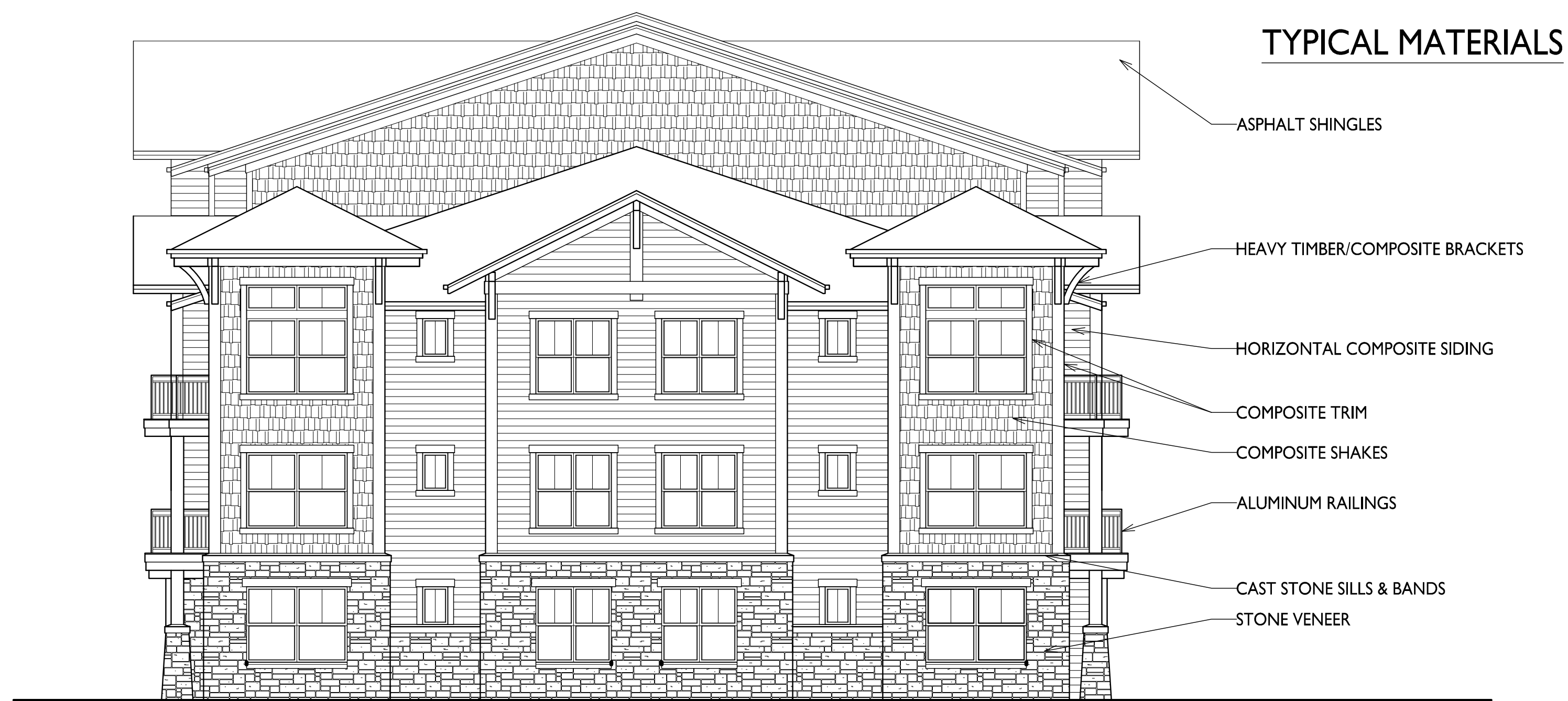
BUILDING 2/CLUBHOUSE NORTHEAST ELEVATION 1/8"=1'-0"
