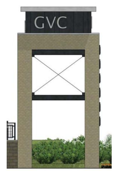
⑩ SIGNAGE TOWER WEST ELEVATION 3/16" = 1'-0"
