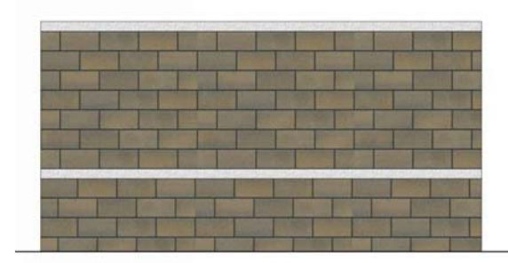
⑬ TRASH ENCLOSURE SIDE & BACK ELEVATION 3/8" = 1'-0"
