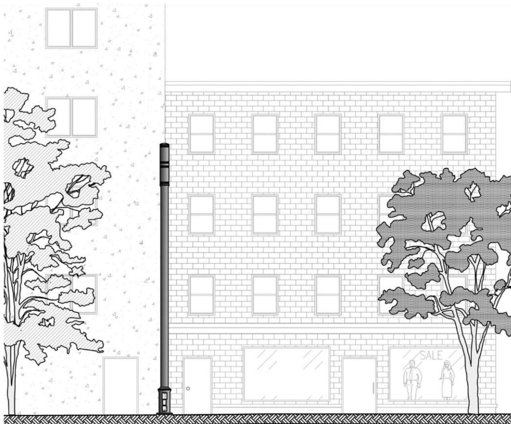
Figure 5-3.4: Small Cell in Commercial Area
