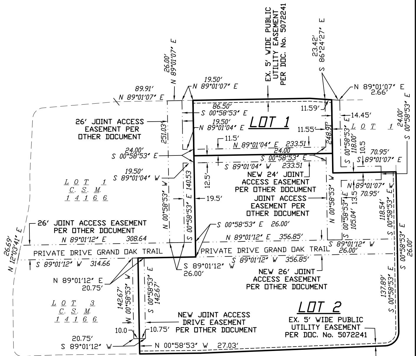
BEARINGS ARE REFERENCED TO THE EAST LINE OF THE NW 1/4 OF SECTION 9-7-10, LINE TO BEAR S 0°58'53" E
