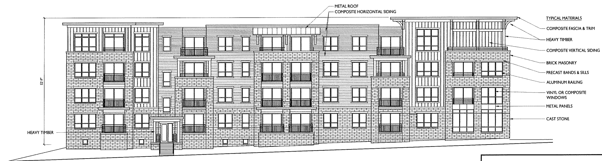
2 WEST ELEVATION ALONG COMMERCE DRIVE A-2.1 3/32" = 1'-0"
