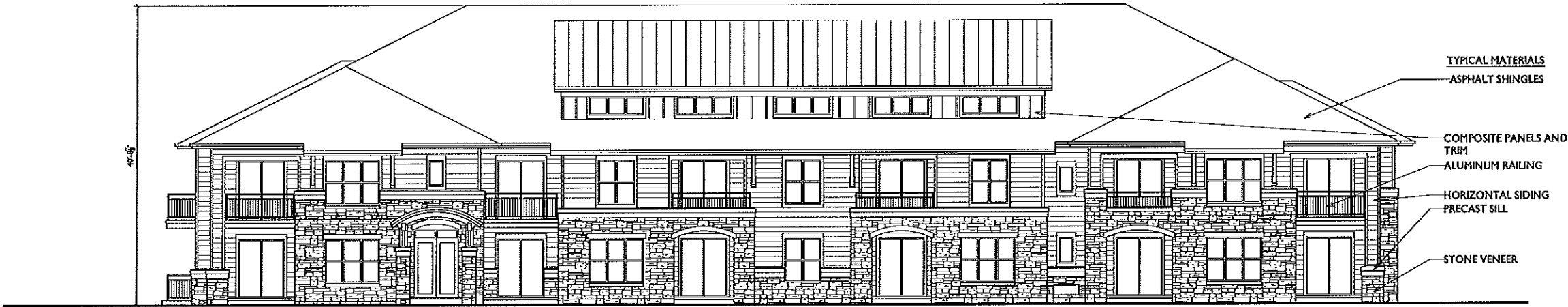
1 EAST ELEVATION - BUILDING I 5 SCALE: 1/8"=1'-0"
