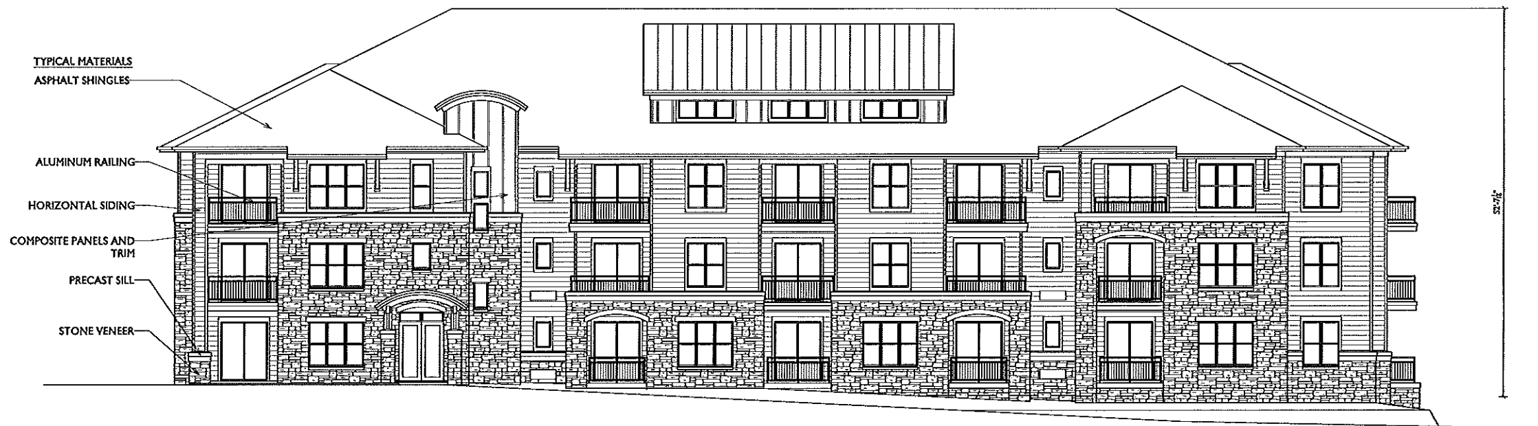
2 NORTH ELEVATION - BUILDING 10 9 SCALE: 1/8"=1'-0"
