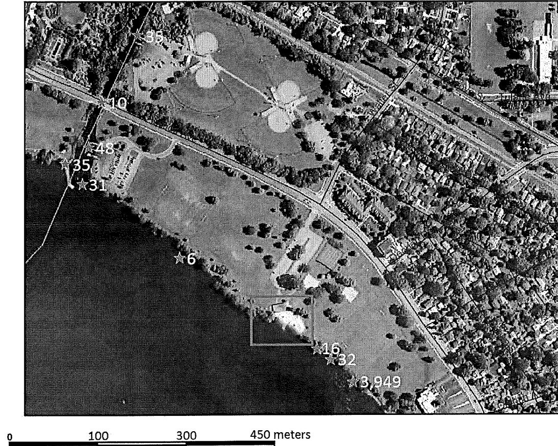
Figure 5: Geometric mean of RHD sampling results. The stormwater outfall is designated by red star at the far right of the figure. Results for the area highlighted by the red square are in Figure 6.
