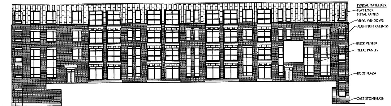
2 COURTYARD ELEVATION A-2.2 1/16"=1'-0"
