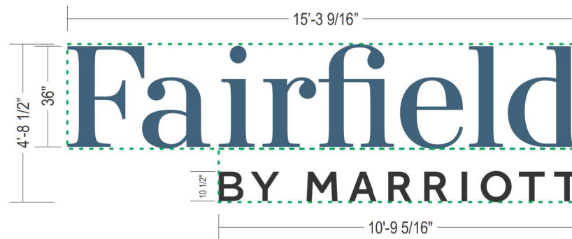
CHANNEL LETTER DETAIL SCALE: 1/4" = 1'-0"
