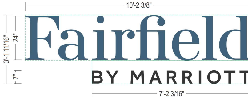
CHANNEL LETTER DETAIL SCALE: 3/8" = 1'-0"
