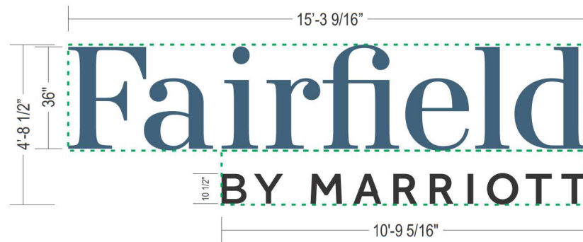
CHANNEL LETTER DETAIL SCALE: 1/4" = 1'-0"
