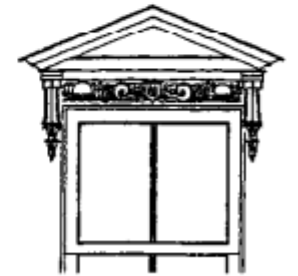
Tin or zinc pedimented hood
