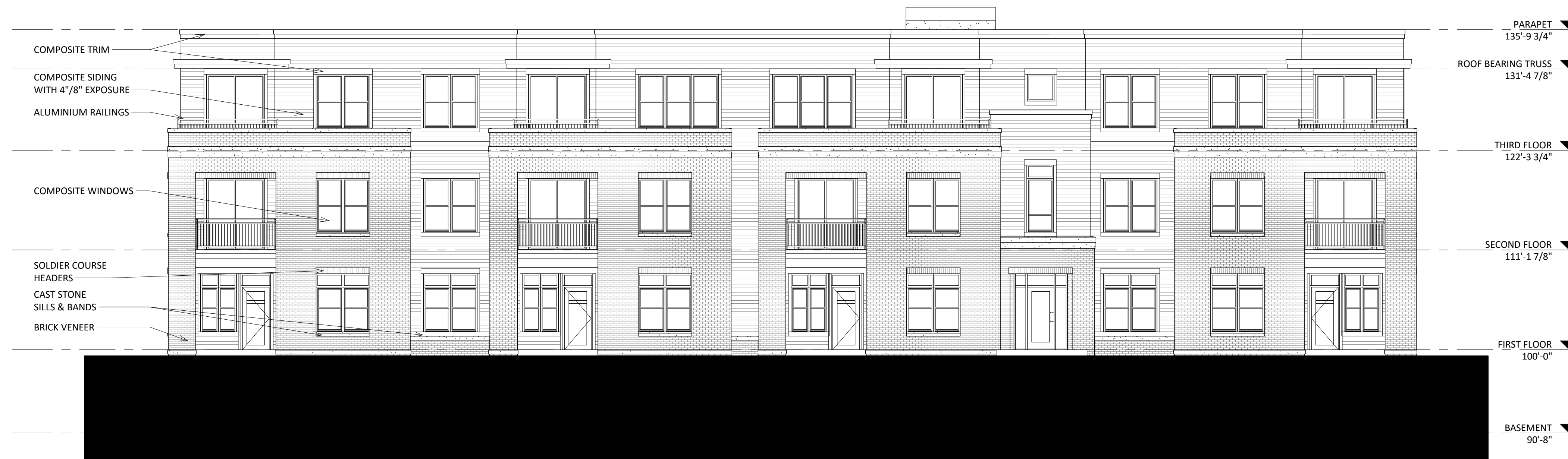
1 ELEVATION - NORTH A-2.1 1/8" = 1'-0"
