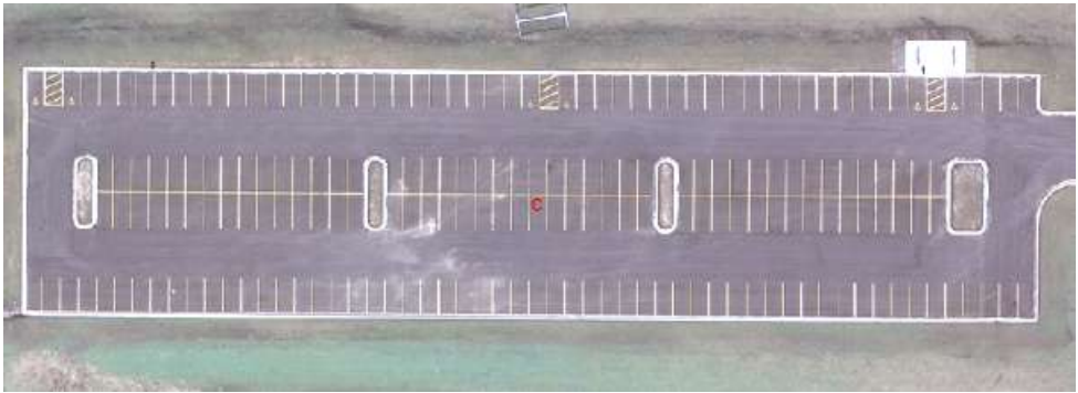
2% Landscaped Coverage within Interior of Parking Lot
