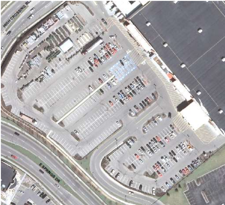
4% Landscaped Coverage within Interior of Parking Lot
