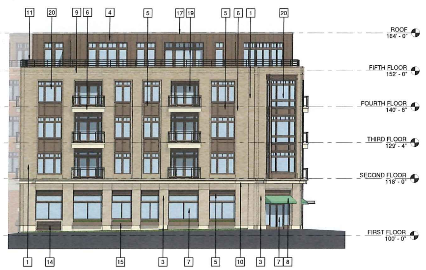
4 Spooner Street (West) Elevation A201 3/32" = 1'-0"
