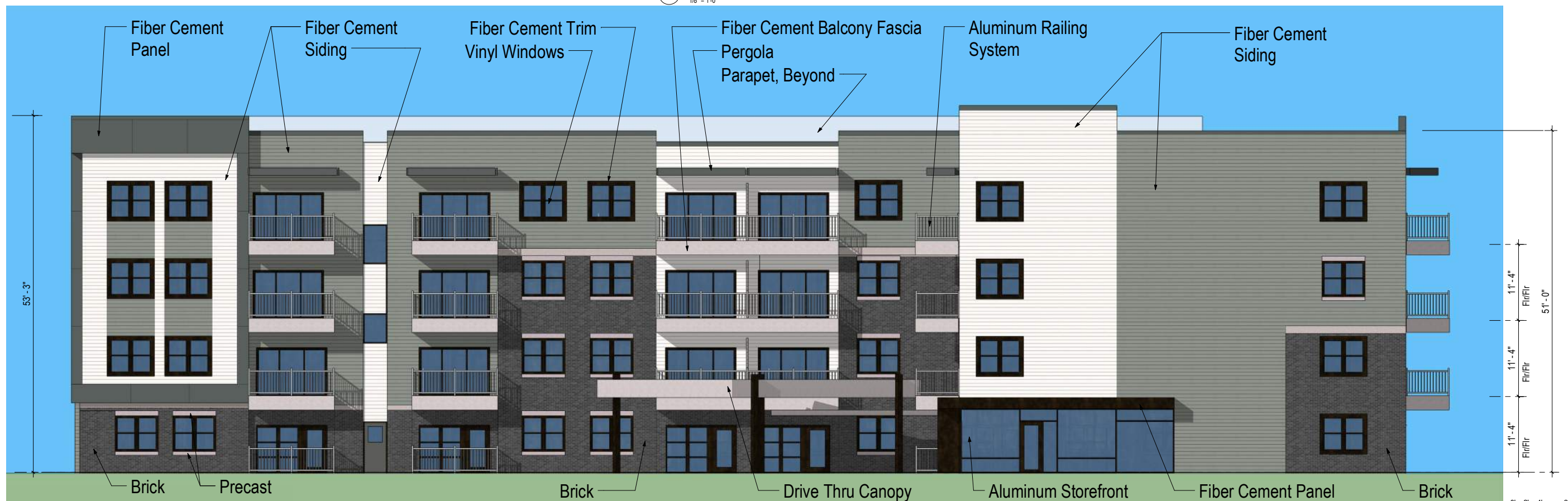
② Sr Building East Elevation 1/8" = 1'-0"
