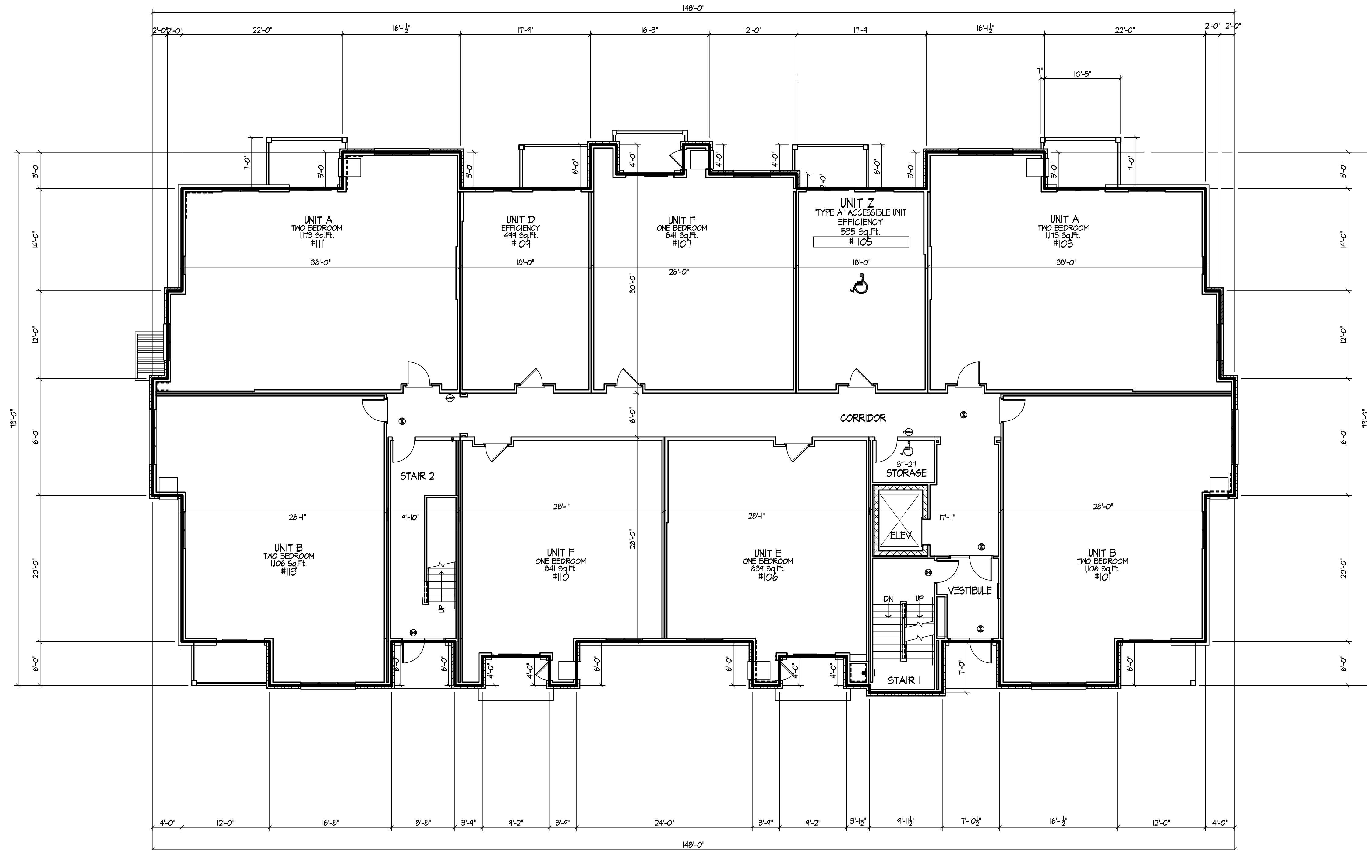
FIRST FLOOR PLAN 9491 S.F. 1/8" = 1'-0"
