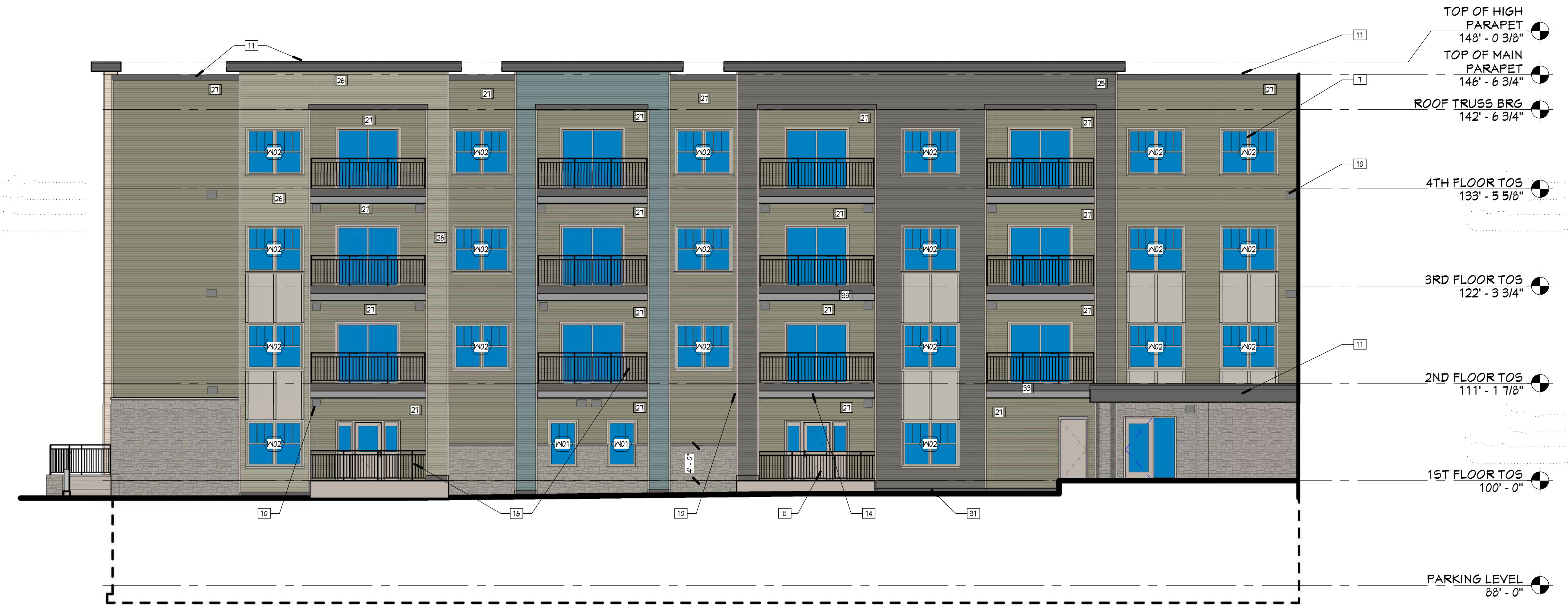
1 PARTIAL NORTH ELEVATION - BUILDING 1 - PROPOSED DESIGN PR1.6 1/8" = 1'-0" BUILDING 1 - ZONE A SHOWN BUILDING 2 - ZONE C SIMILAR
