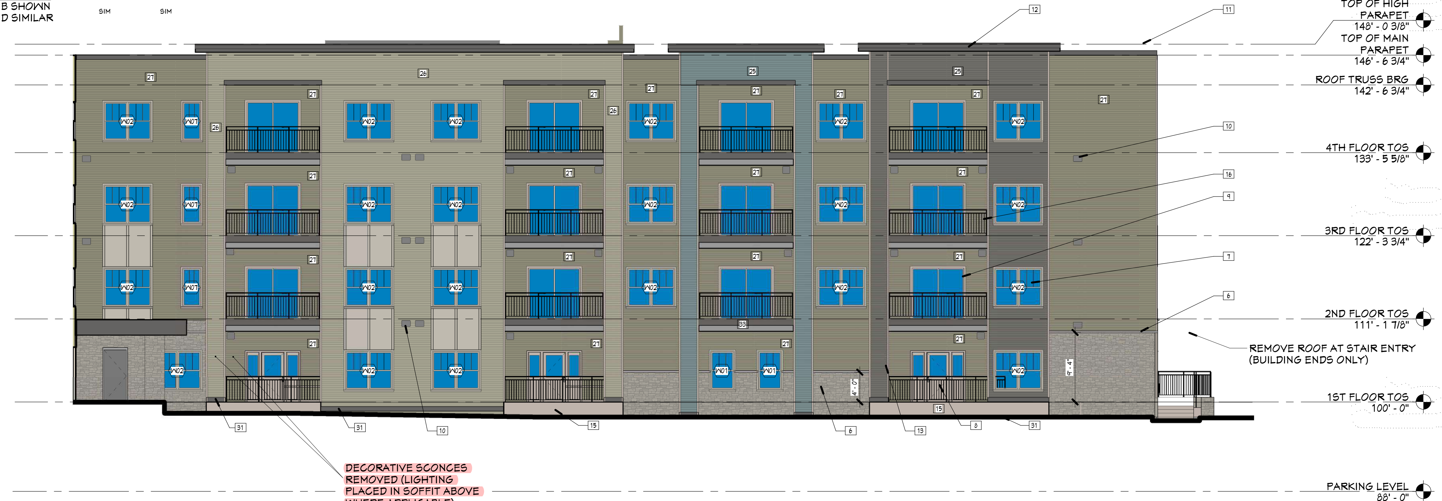
3 PARTIAL EAST ELEVATION - BLDG 1 - PROPOSED DESIGN BUILDING 1 - ZONE B SHOWN BUILDING 2 - ZONE D SIMILAR PR1.4 1/8" = 1'-0"
