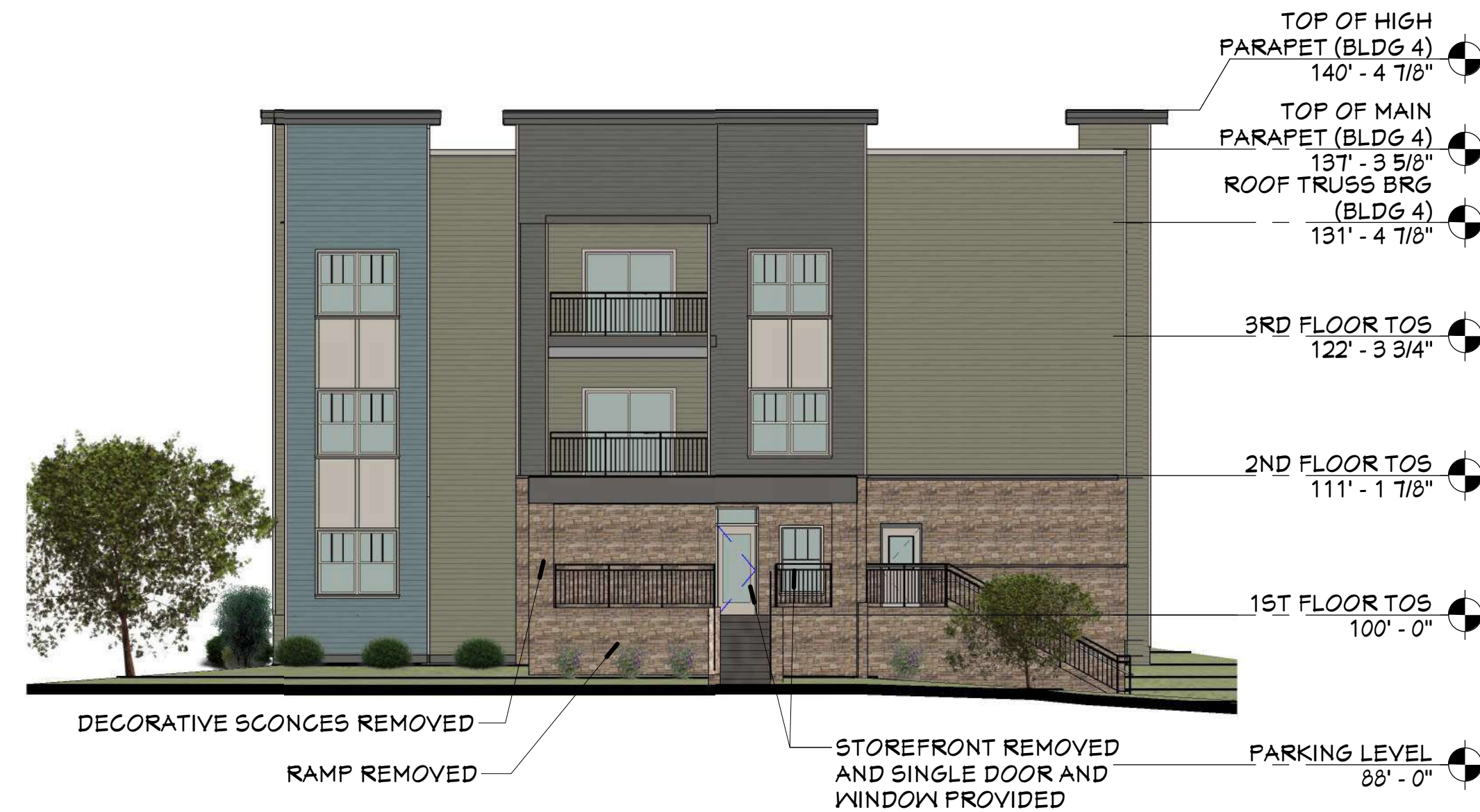
3 NORTHWEST ELEVATION - BUILDING 4 - PROPOSED CHANGES PR3.2 3/9/21 = 1'-0"
