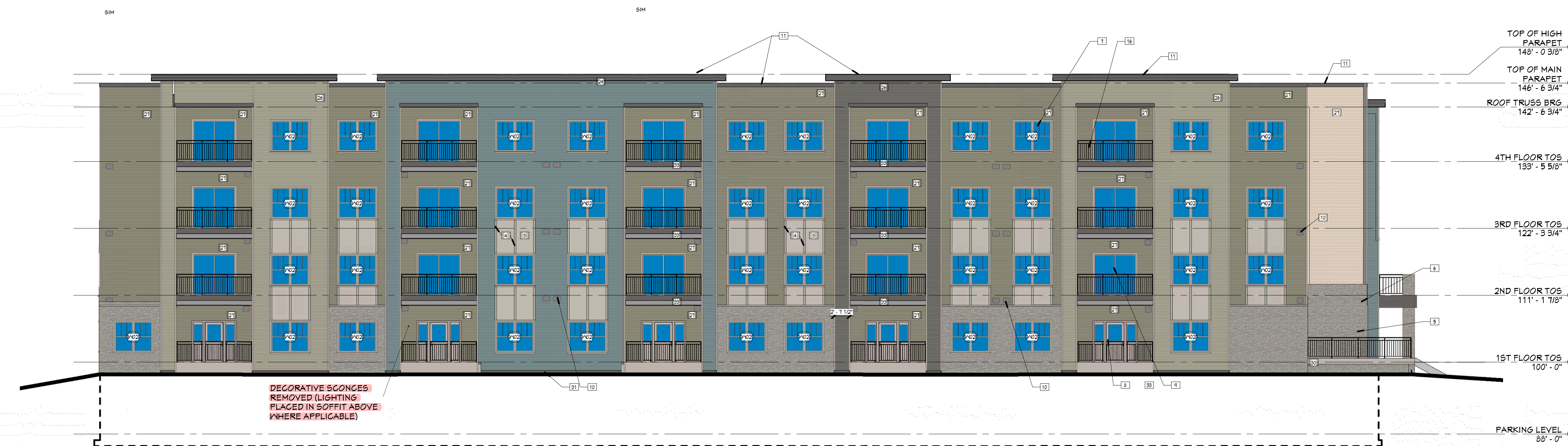
1 WEST ELEVATION - BUILDING 1 - PROPOSED DESIGN 1/8" = 1'-0" BUILDING 1 - ZONE B SHOWN BUILDING 2 - ZONE D SIMILAR
