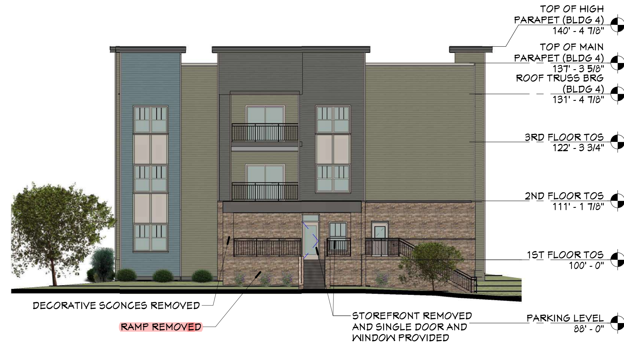
3 NORTHWEST ELEVATION - BUILDING 4 - PROPOSED CHANGES PR3.2 3/9/21 = 1'-0"
