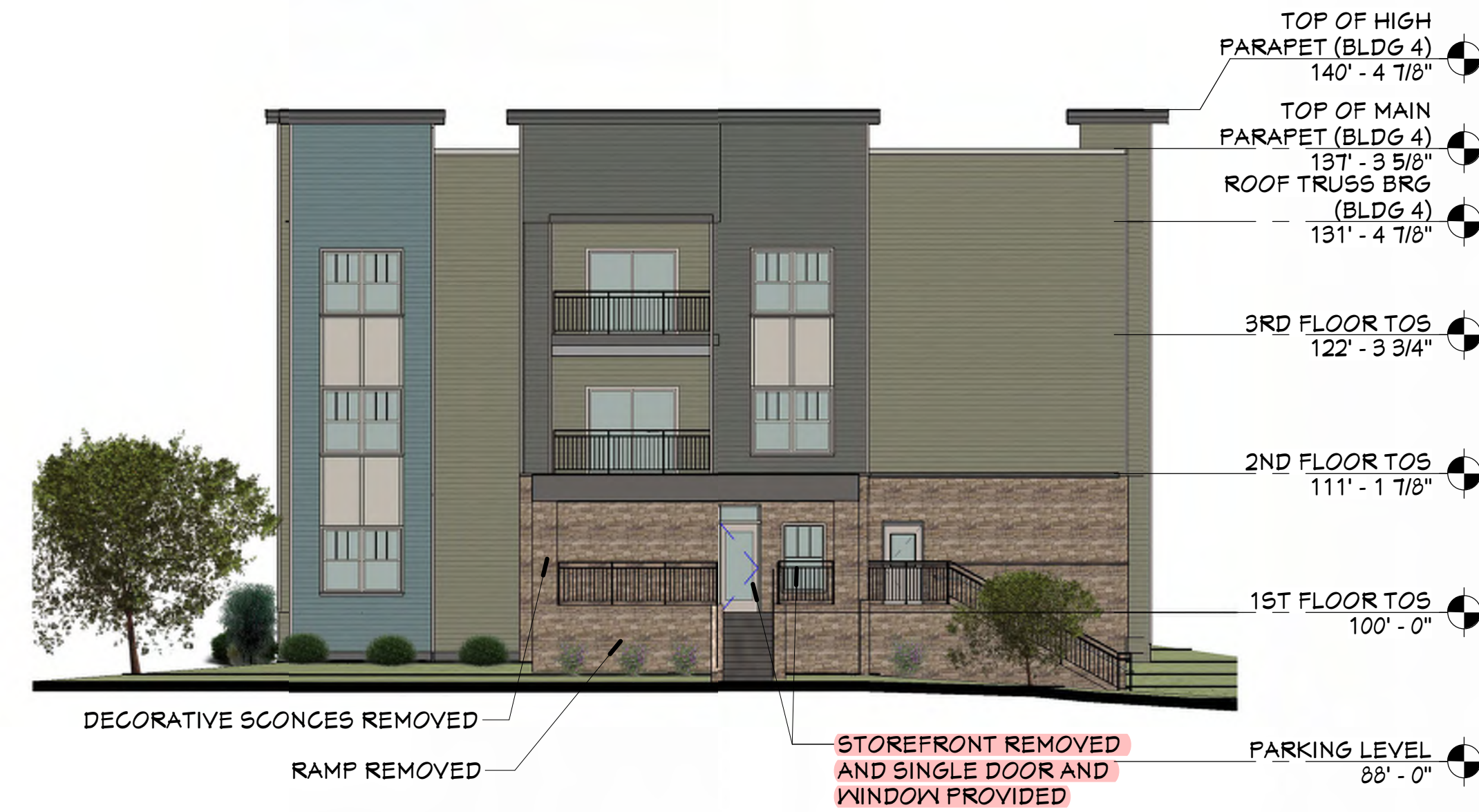
3 NORTHWEST ELEVATION - BUILDING 4 - PROPOSED CHANGES PR3.2 3/9/21 = 1'-0"
