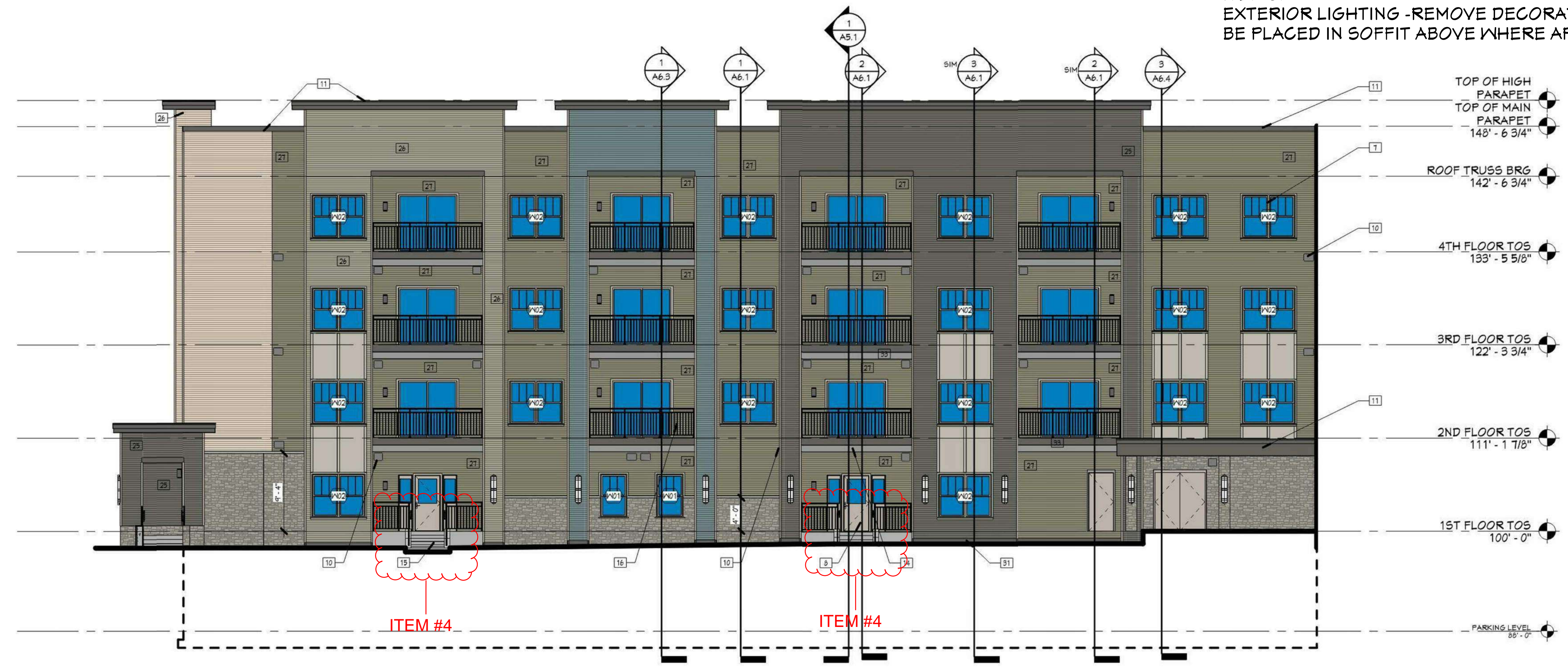
2 PARTIAL NORTH ELEVATION - BLDG 1 - CURRENT APPROVED DESIGN PR1.6 1/8" = 1'-0" BUILDING 1 - ZONE A SHOWN BUILDING 2 - ZONE C SIMILAR
