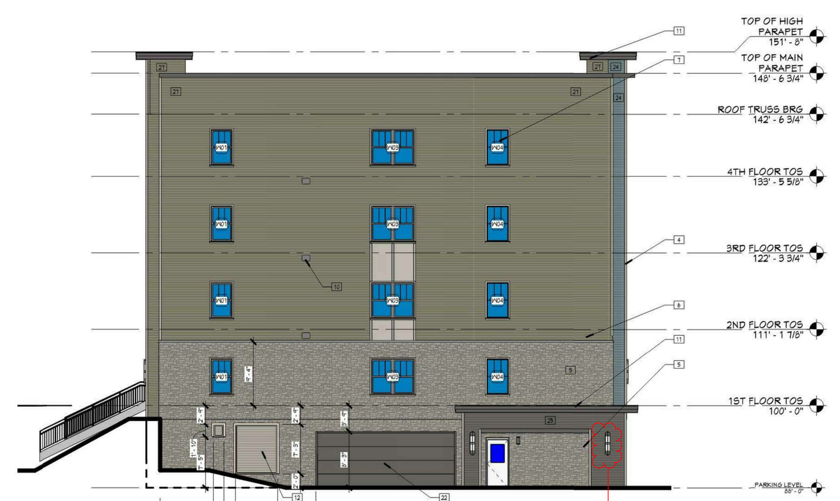
3 SOUTH ELEVATION - BLDG 3 - CURRENT APPROVED DESIGN PR2.3 1/8" = 1'-0"
