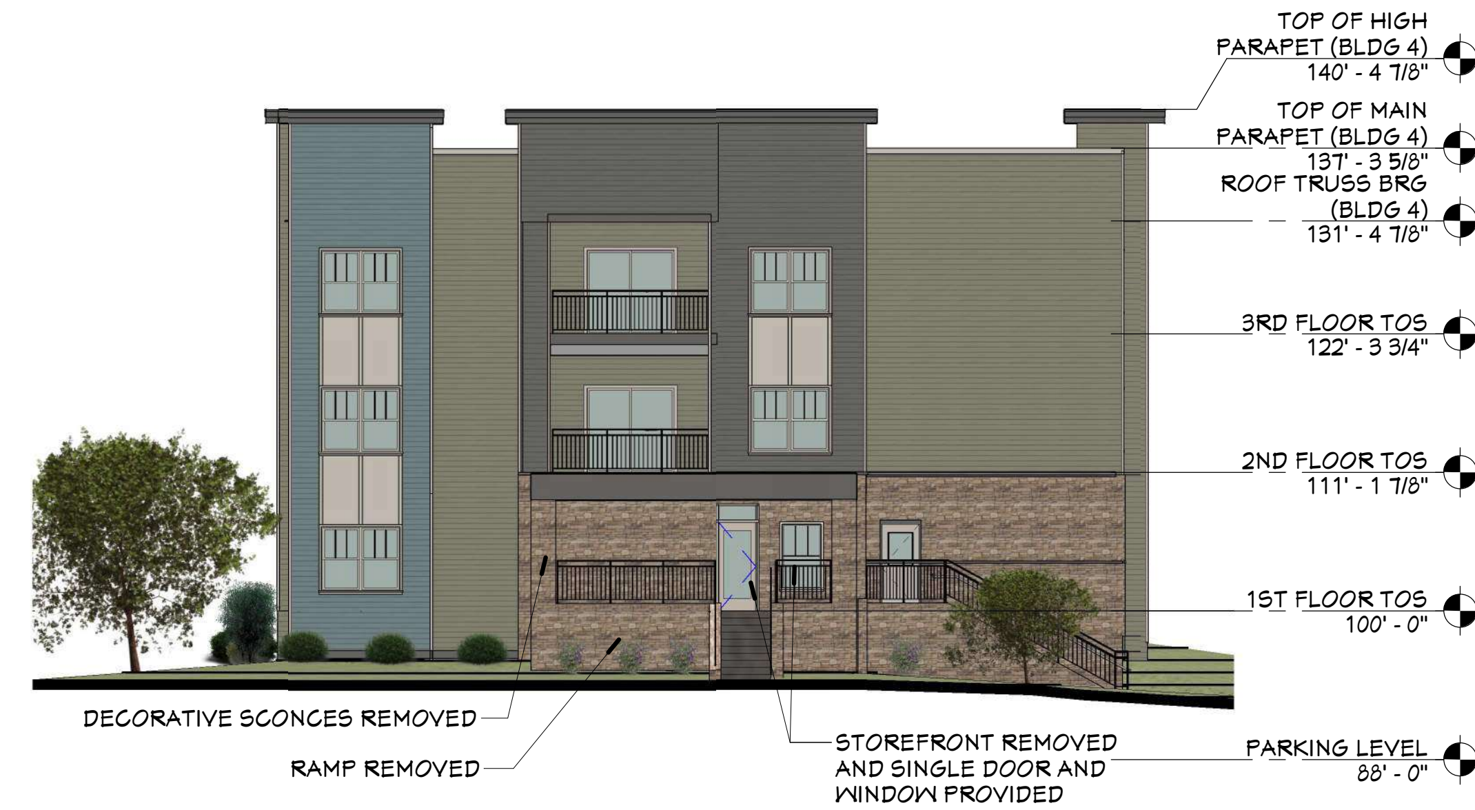
3 NORTHWEST ELEVATION - BUILDING 4 - PROPOSED CHANGES PR3.2 3/9/21 = 1'-0"
