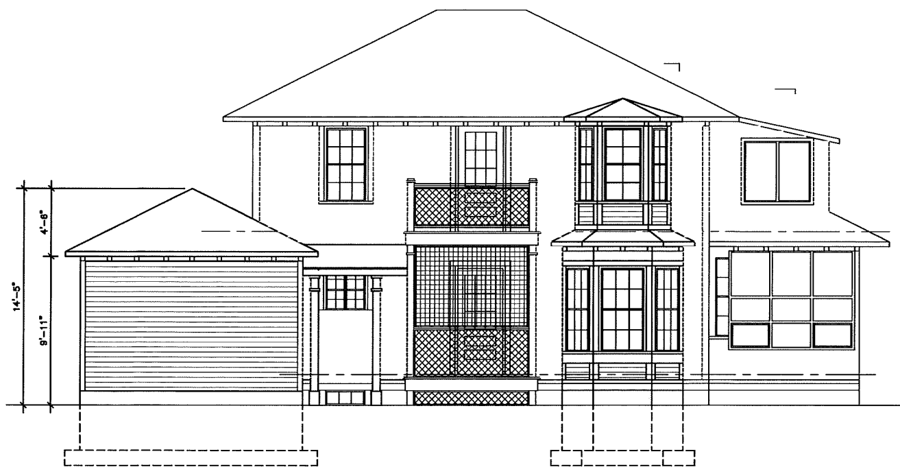
3 WEST EXTERIOR ELEVATION 1/4"=1'-0"
