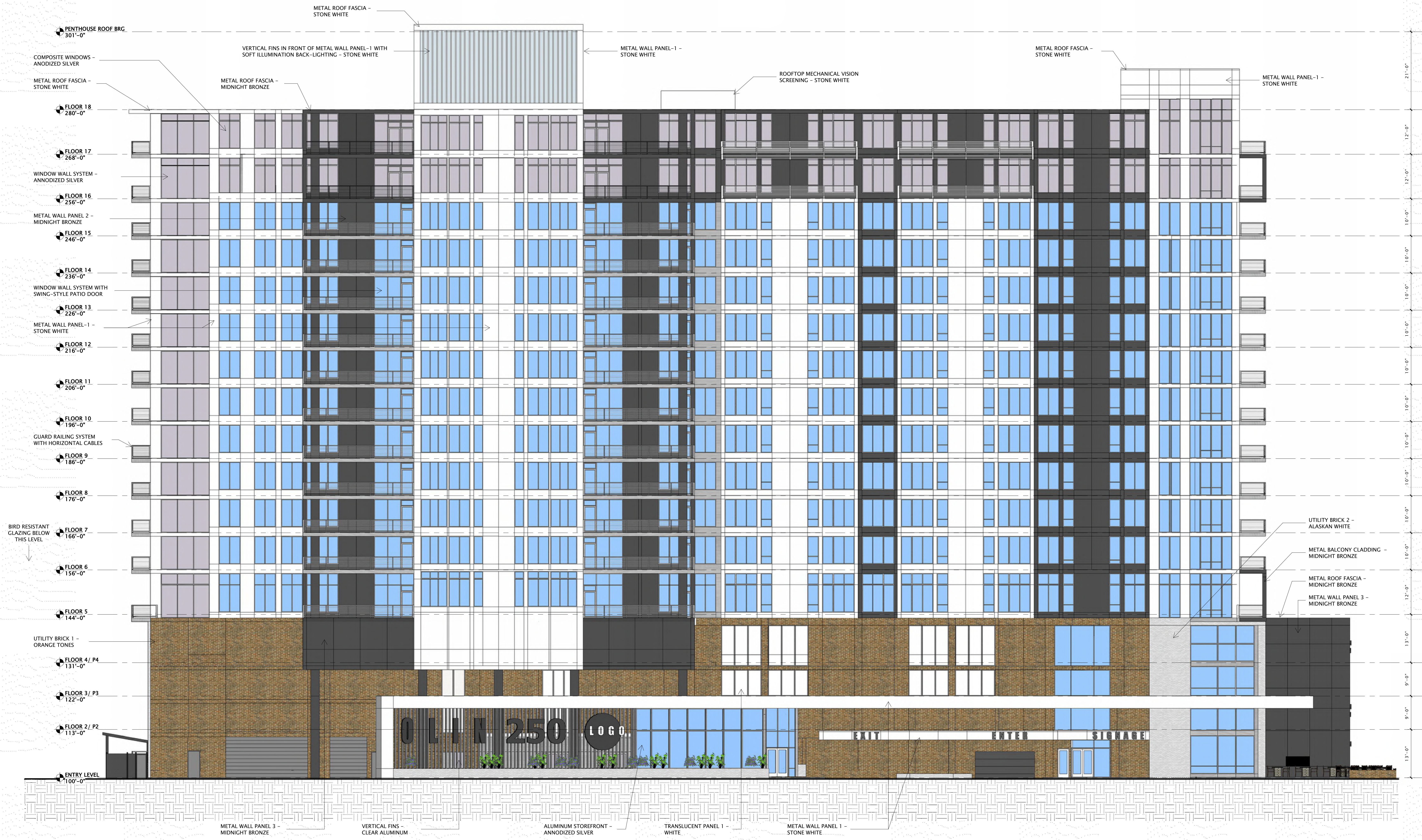
25 SOUTH EXTERIOR ELEVATION 3/32" = 1'-0"
