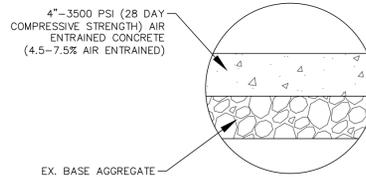
CONCRETE SIDEWALK SECTION
