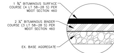
ASPHALT PAVEMENT SECTION
