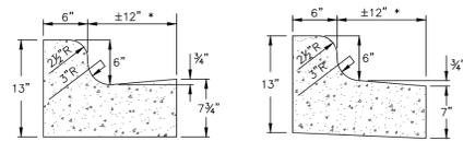
18" STANDARD CONCRETE CURB & GUTTER
