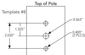
DSX1 shares a unique drilling pattern with the AERIS™ family. Specify this drilling pattern when specifying poles, per the table below.
