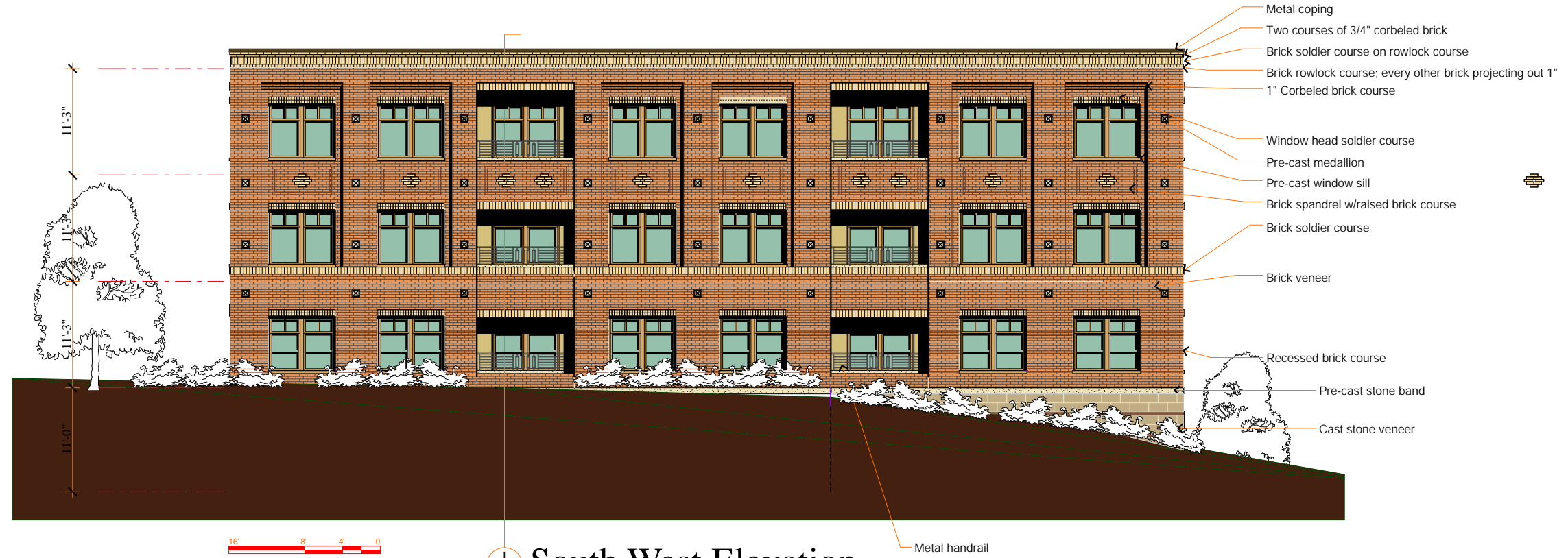
South West Elevation
