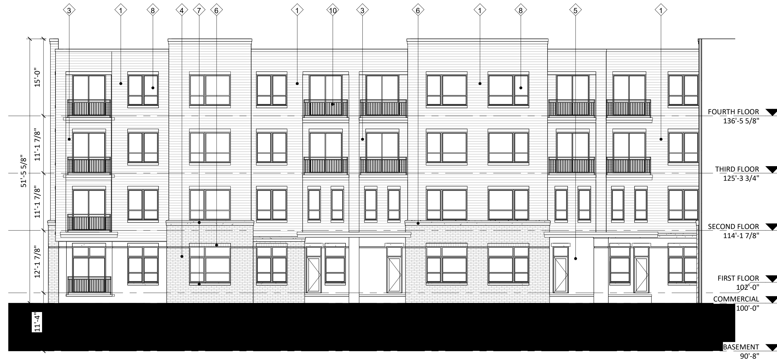
1 ELEVATION - EAST INTERIOR A203 3/32" = 1'-0"
