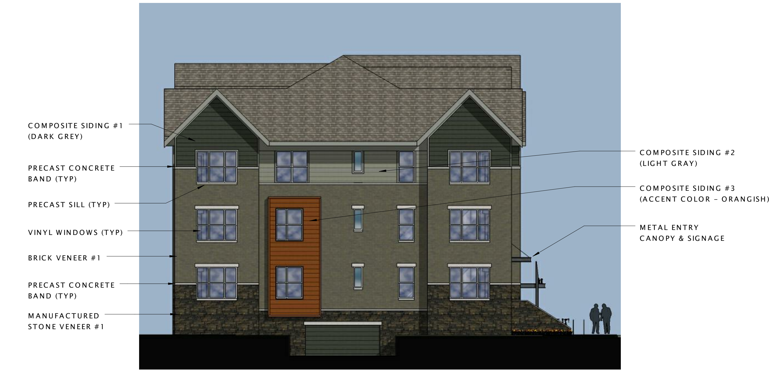
16 TYPICAL 'B' BUILDING - END ELEVATION (W/ GARAGE) 3/32" = 1'-0"
