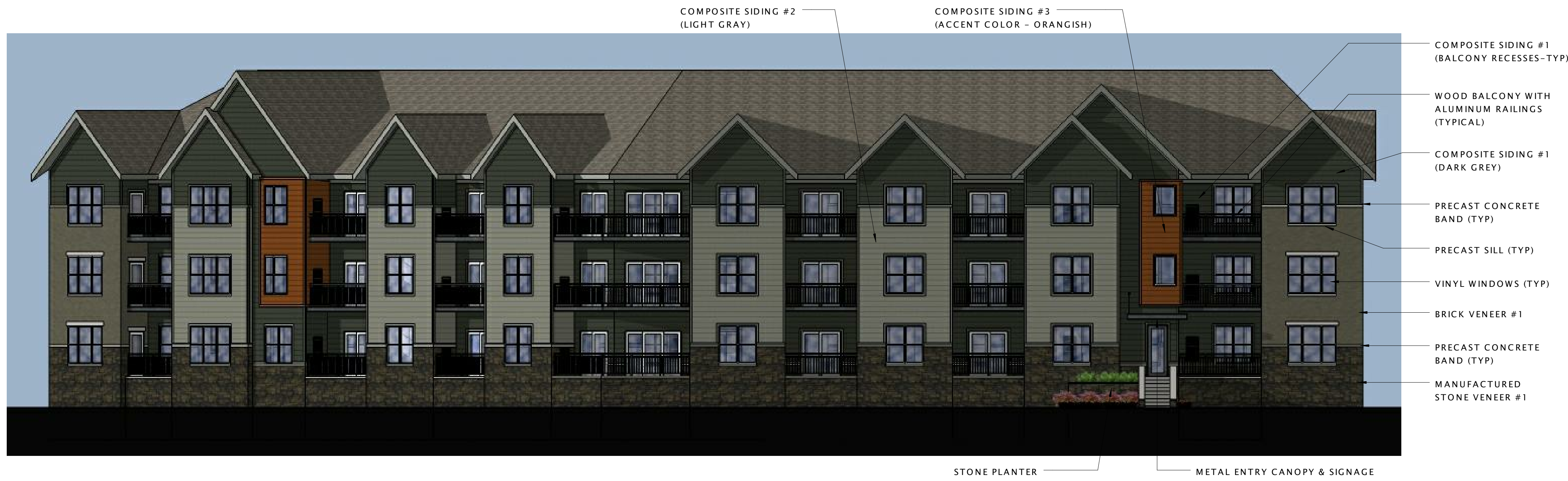
6 TYPICAL 'B' BUILDING - REAR ELEVATION #1 3/32" = 1'-0"
