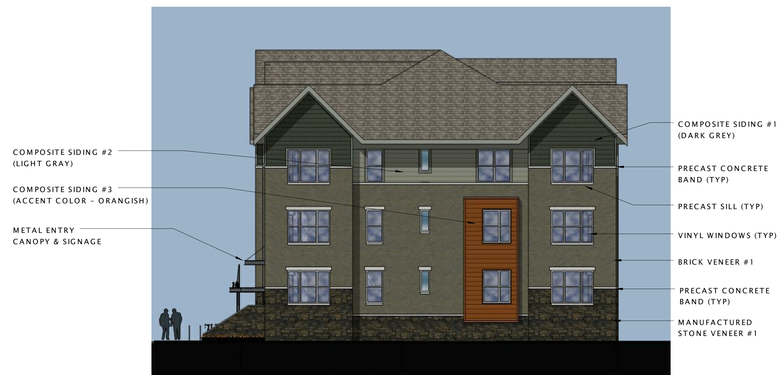
⑪ TYPICAL 'A' BUILDING - END ELEVATION 3/32" = 1'-0"
