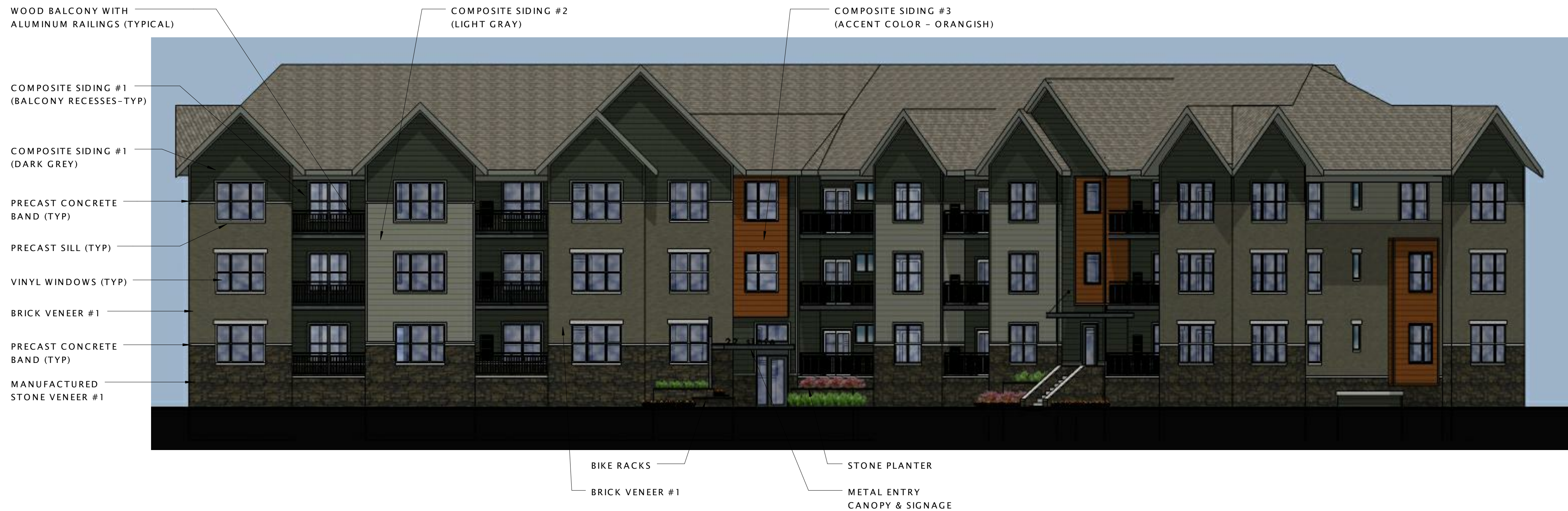
6 TYPICAL 'B' BUILDING - FRONT ELEVATION #1 3/32" = 1'-0"
