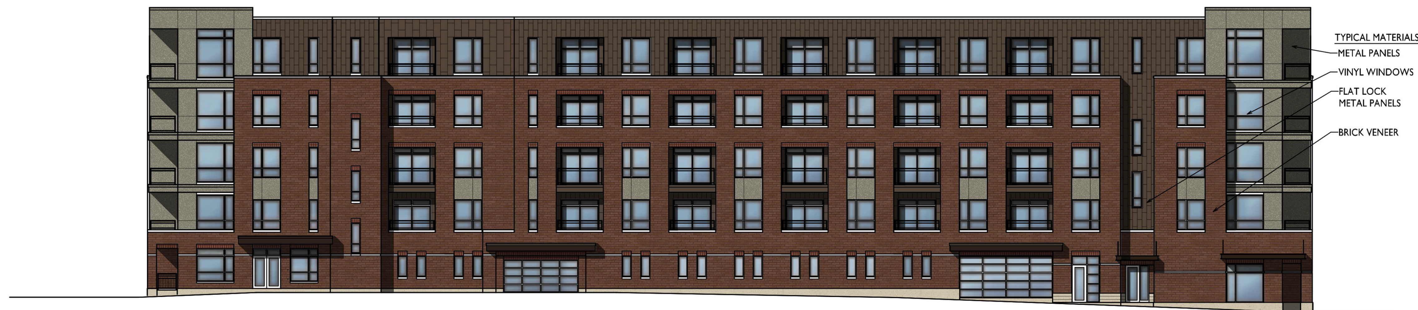
4 SOUTH ELEVATION A-2.2 1/16"=1'-0"
