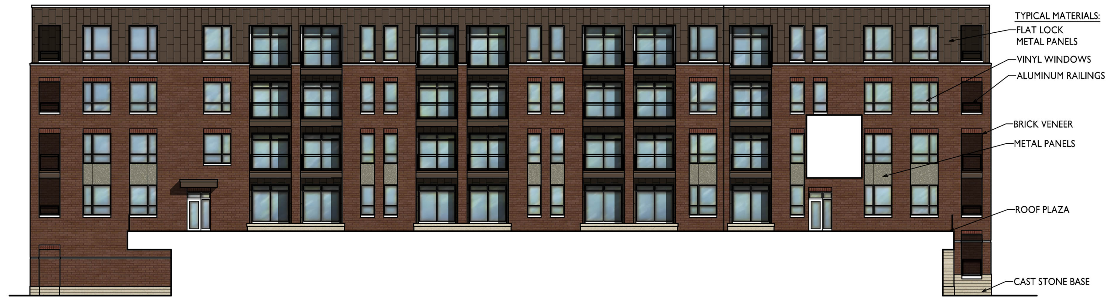
2 COURTYARD ELEVATION A-2.2 1/16"=1'-0"
