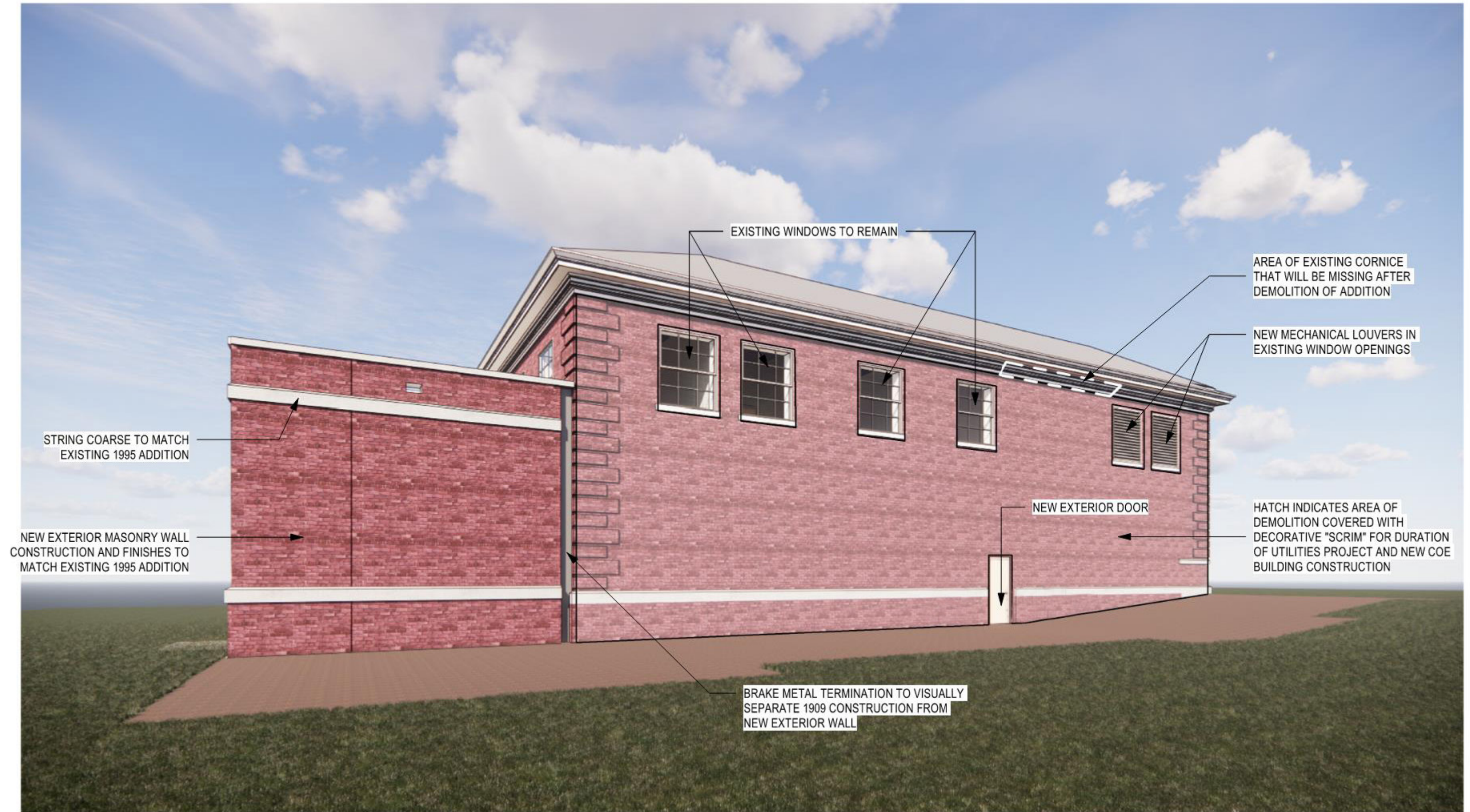
3D RENDERING OF EAST FACADE OF MSE BUILDING FOLLOWING DEMOLITION OF ADDITION AND CONSTRUCTION OF NEW EXTERIOR WALL.
