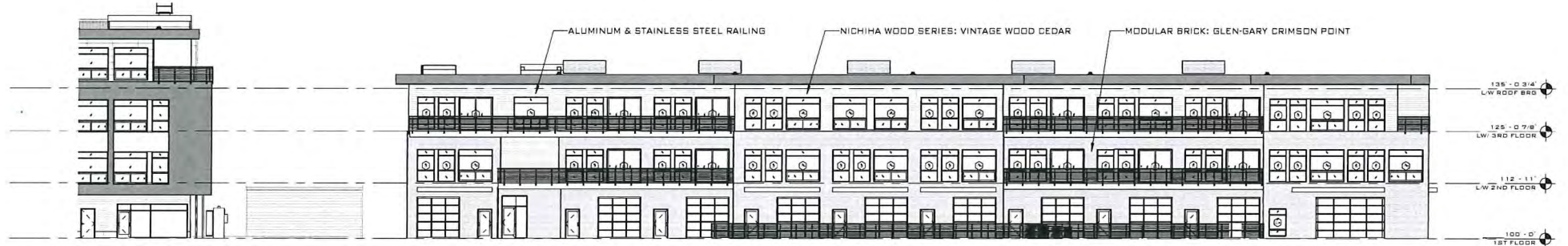
4 LIVE/WORK MIFFLIN ELEVATION 1/16" = 1'-0"
