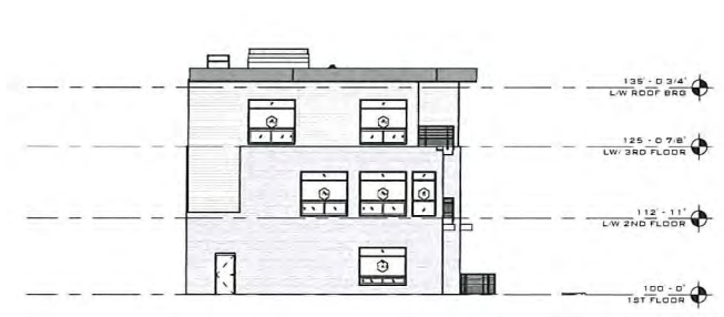
6 LIVE/WORK COURTYARD ELEVATION 1/16" = 1'-0"
