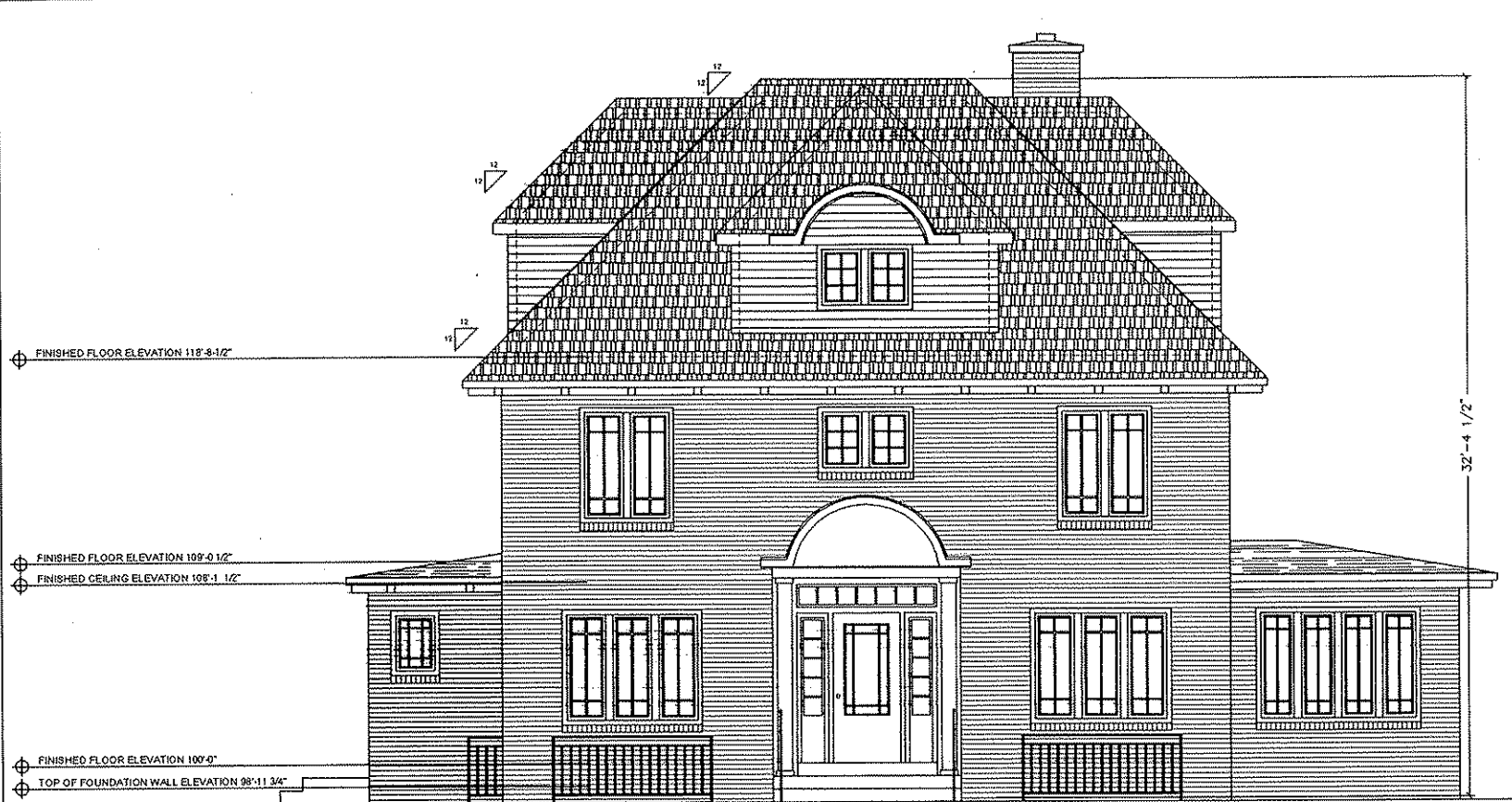
REMODELED WEST EXTERIOR ELEVATION SCALE: 1/8" = 1'-0"
