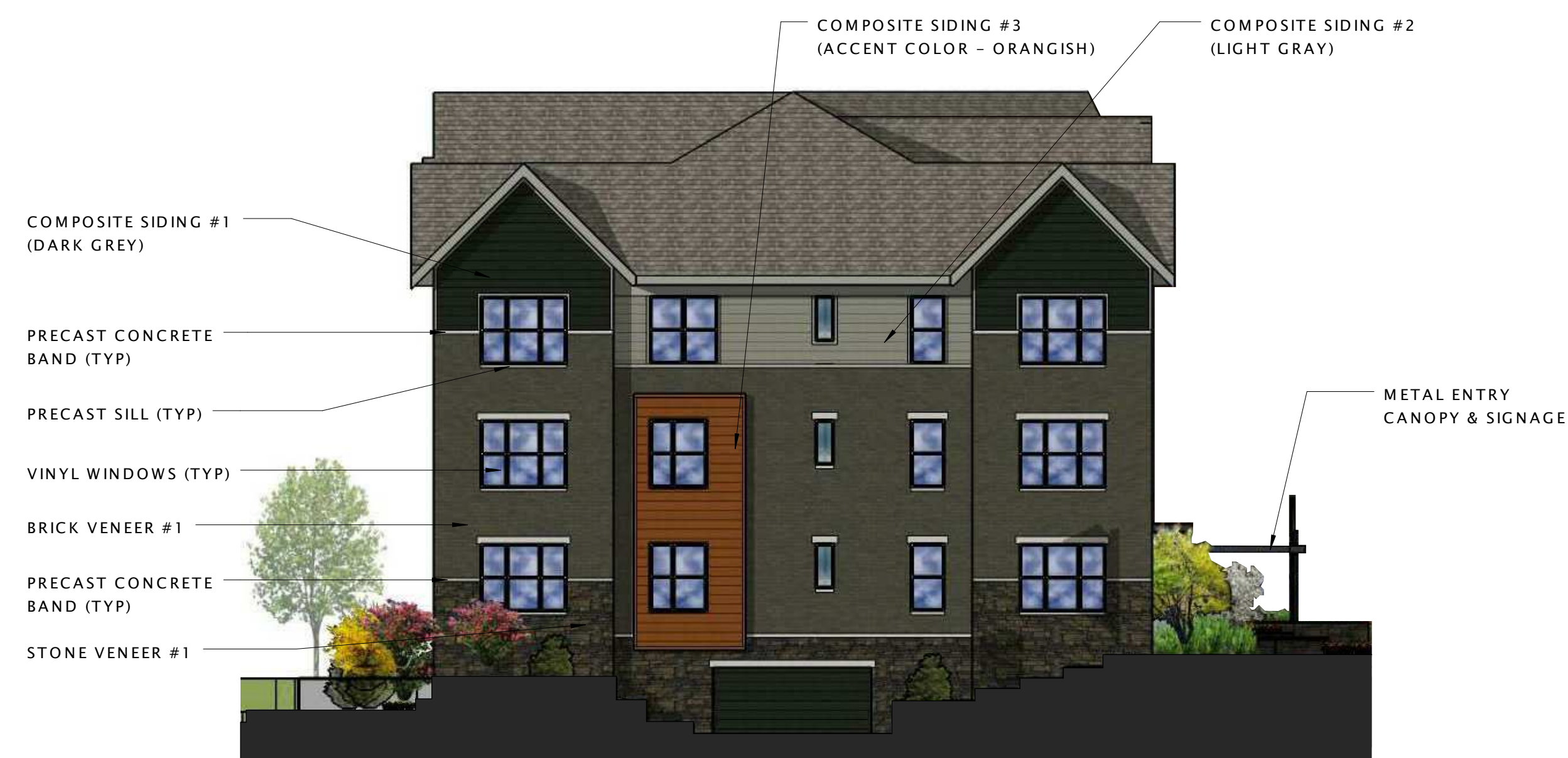
16 B3 & B4 - END ELEVATION (W/ GARAGE) 3/32" = 1'-0"
