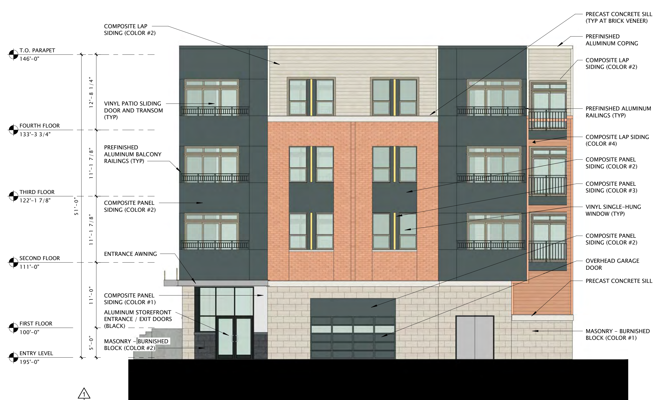
⑩ BUILDING 'C' - WEST ELEVATION 1/8" = 1'-0"
