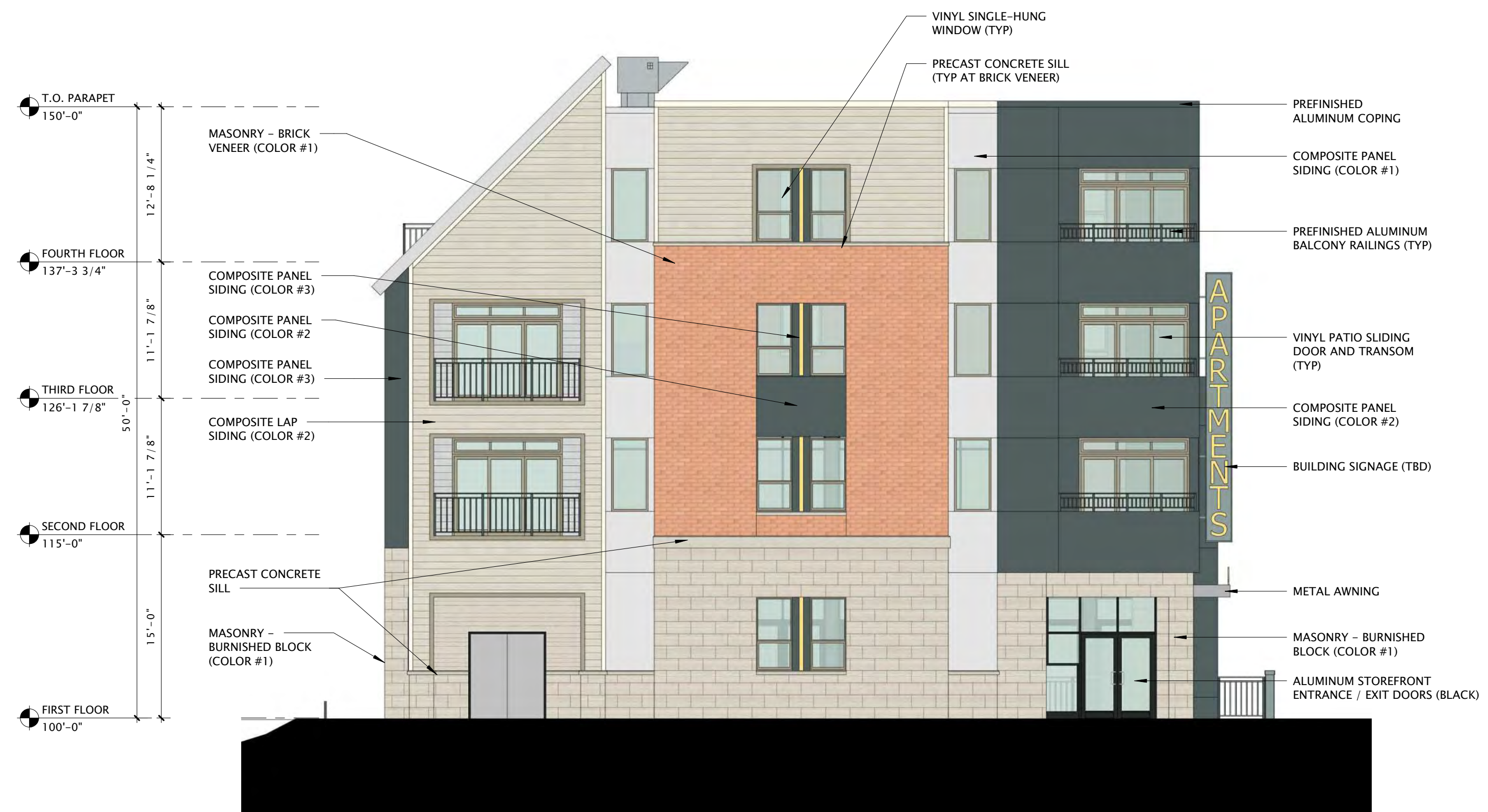
9 BUILDING 'A' - SOUTH ELEVATION 1/8" = 1'-0"
