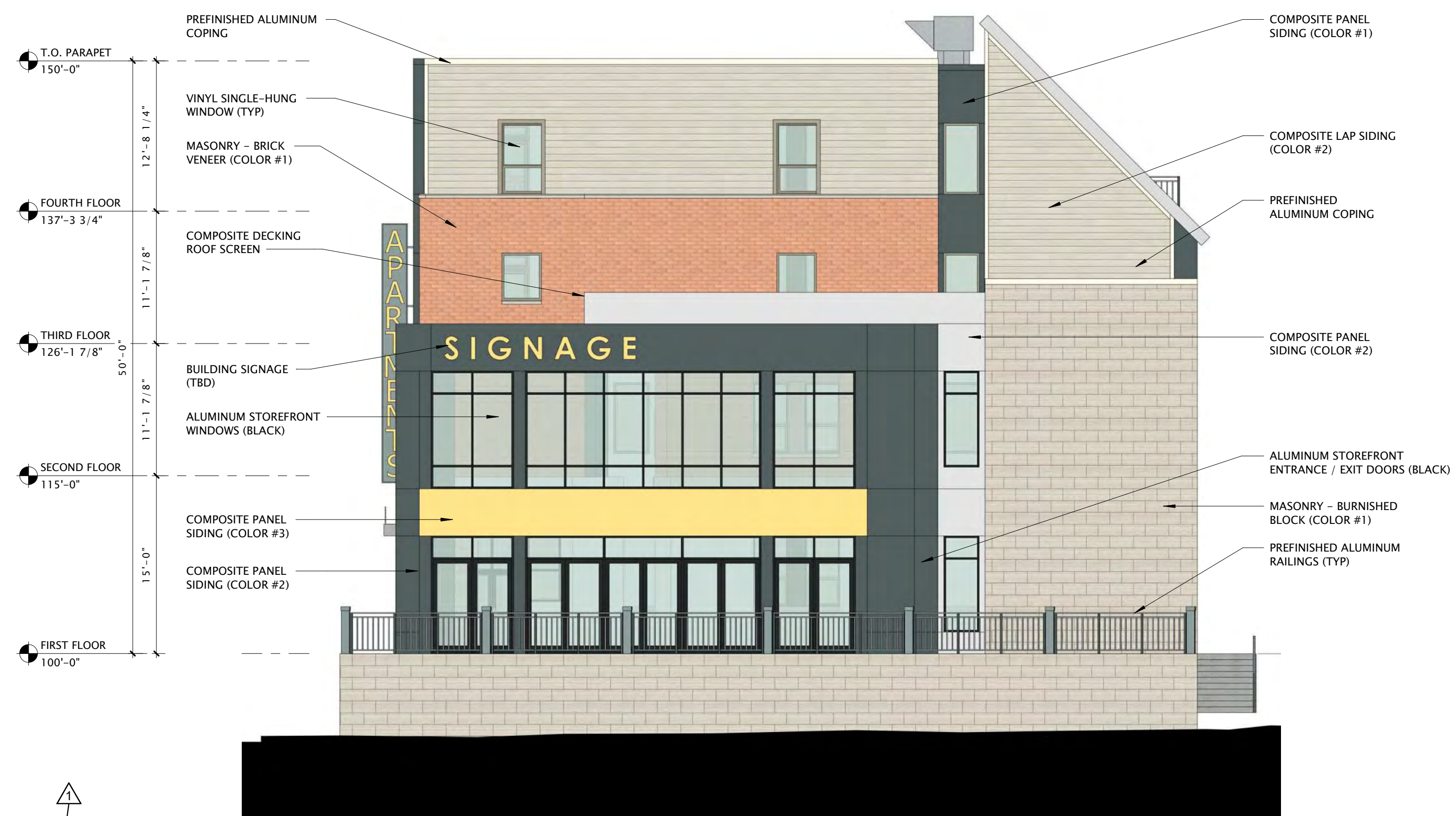
18 BUILDING 'A' - NORTH ELEVATION 1/8" = 1'-0"
