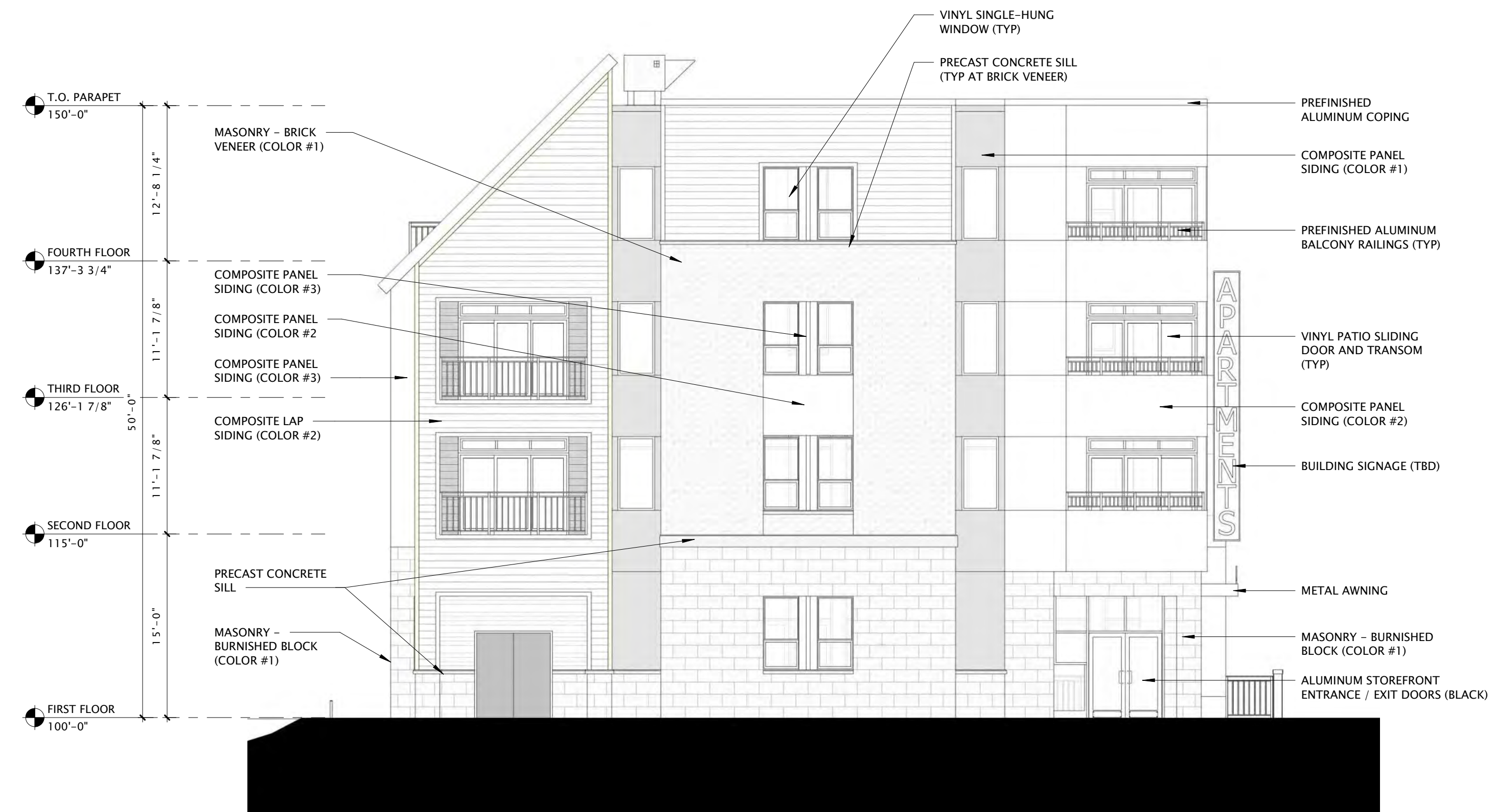
1 BUILDING 'A' - SOUTH ELEVATION BW 1/8" = 1'-0"
