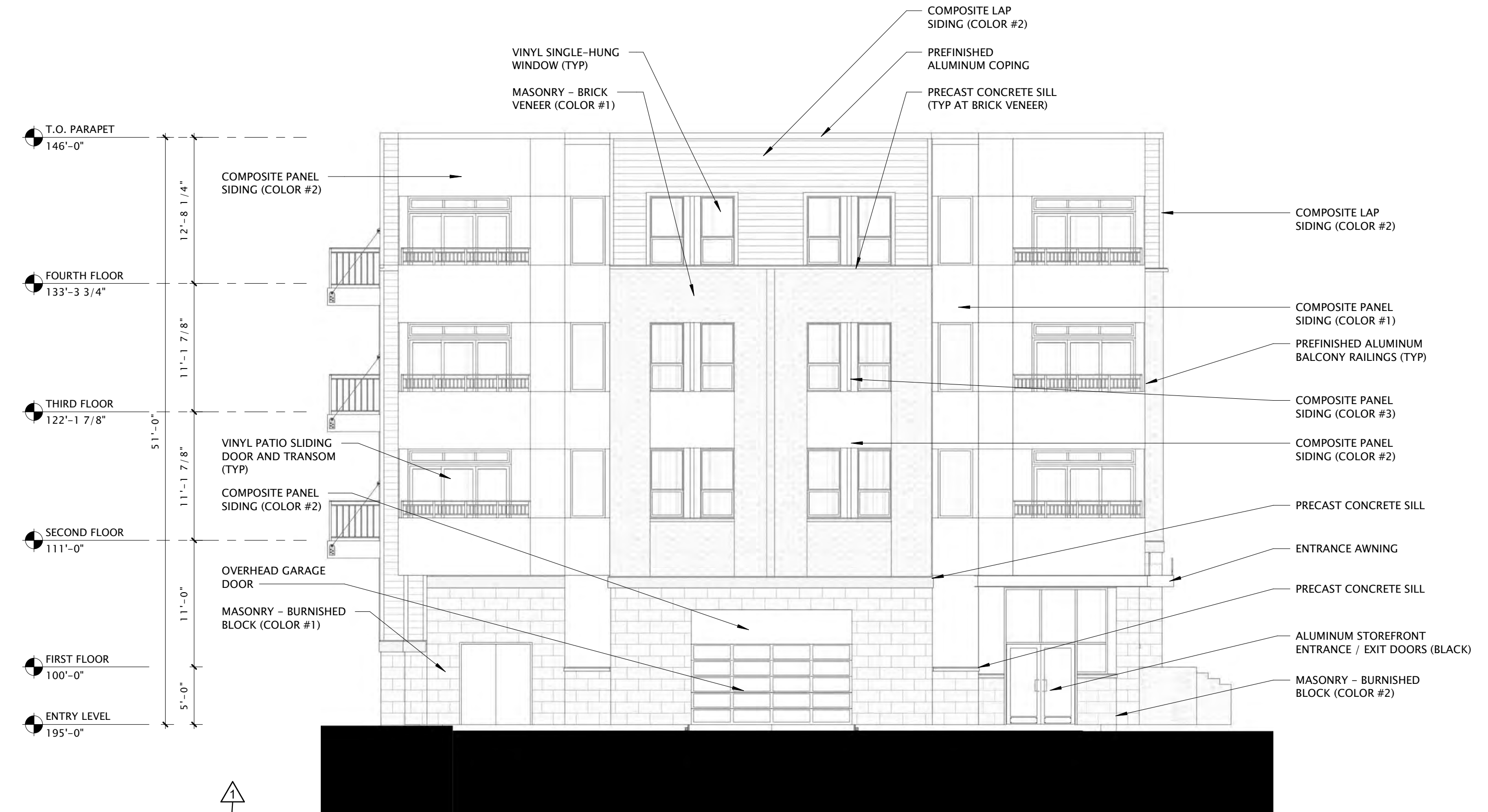
1 BUILDING 'B' - EAST ELEVATION BW 1/8" = 1'-0"
