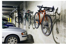
HANGING BIKE RACK DETAIL 66 HANGING BIKE RACKS HAVE BEEN PROPOSED. OF THE 315 BIKES PROVIDED 17.6% ARE PROPOSED TO BE HUNG.
