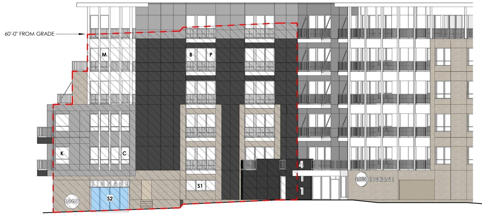
⑦ NORTH ELEVATION BIRD GLASS 1/16" = 1'-0"
