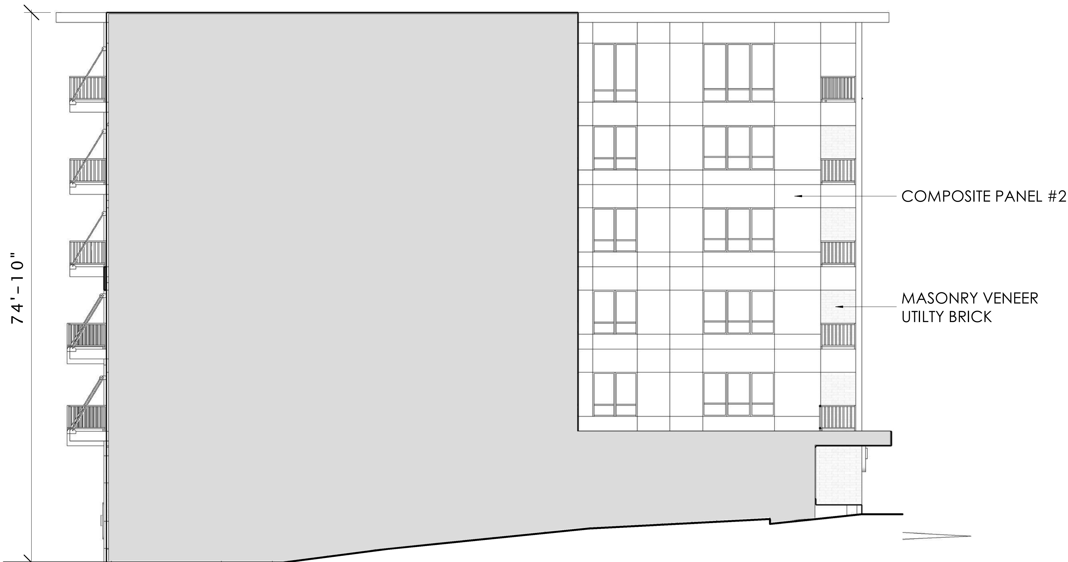
① SOUTHEAST ELEVATION B&W 1/8" = 1'-0"
