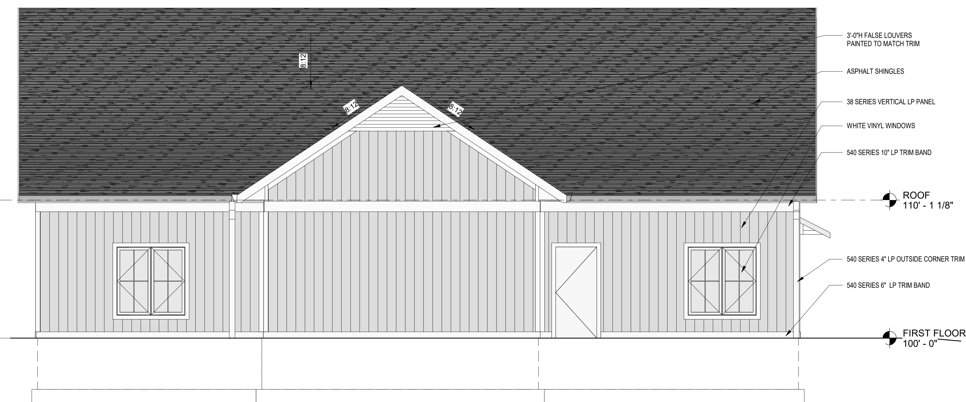
3 SOUTH ELEVATION - CLUBHOUSE A301b SCALE: 1/4" = 1'-0" 0 2' 4' 8' 0 1/4" = 1'-0"
