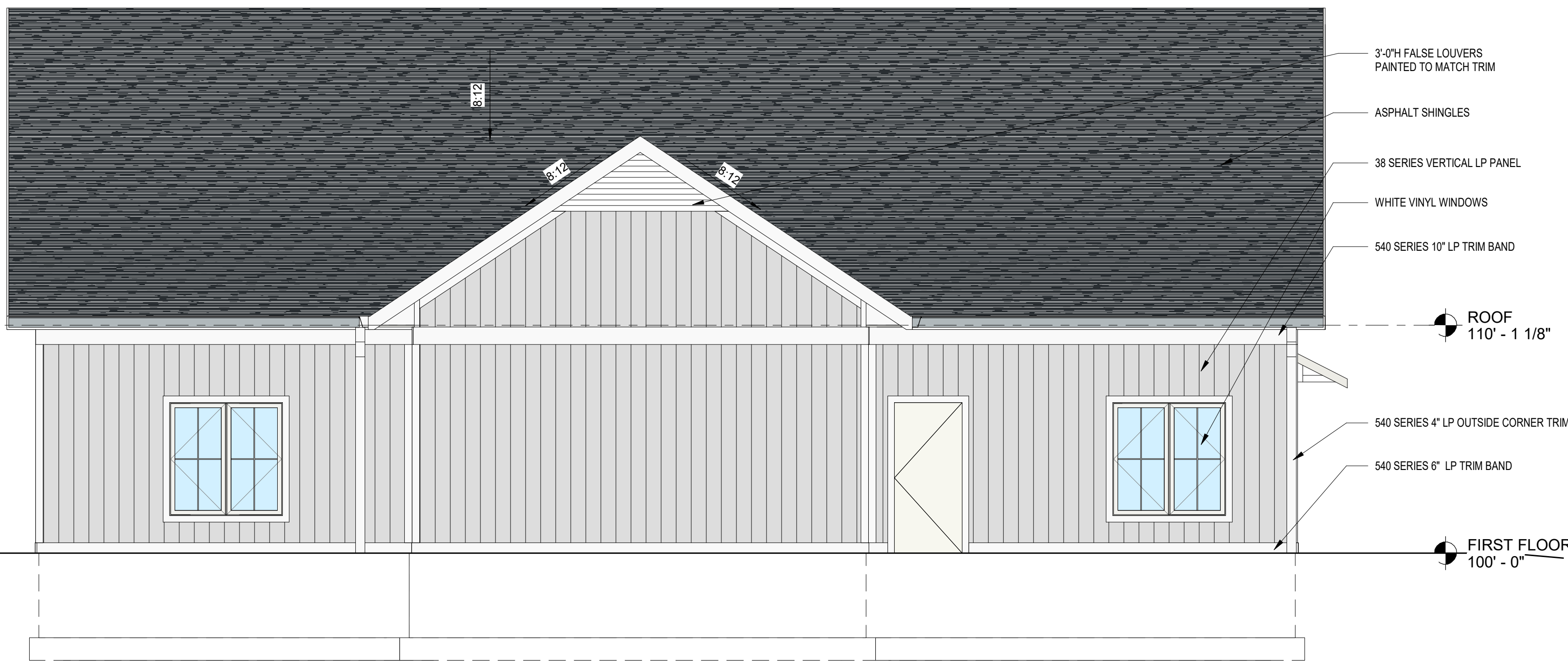
3 SOUTH ELEVATION - CLUBHOUSE A301a SCALE: 1/4" = 1'-0" 0 2' 4' 8' 0 1/4" = 1'-0" 2'
