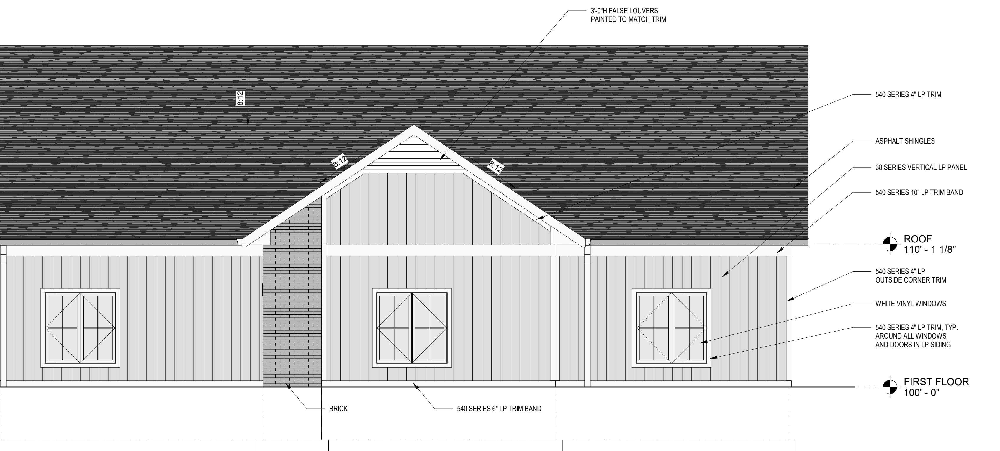
1 NORTH ELEVATION - CLUBHOUSE A301b SCALE: 1/4" = 1'-0" 0 2' 4' 8' 0 1/4" = 1'-0"
