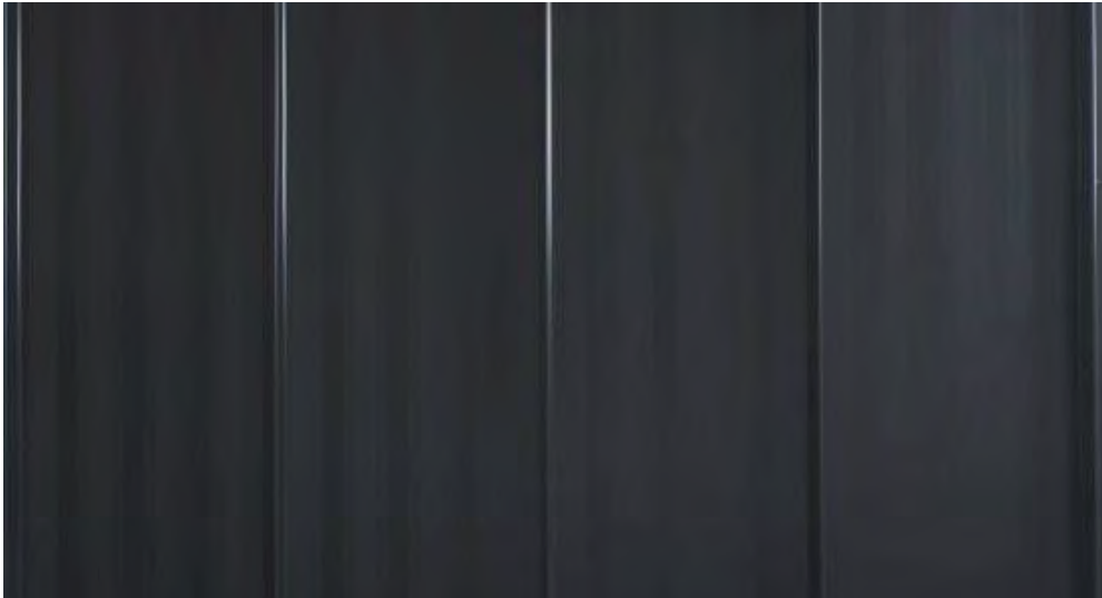
STANDING SEAM METAL PANEL - BLACK (CLADDING IN BETWEEN MASONRY EXPRESSIONS AND UPPER STORY)
