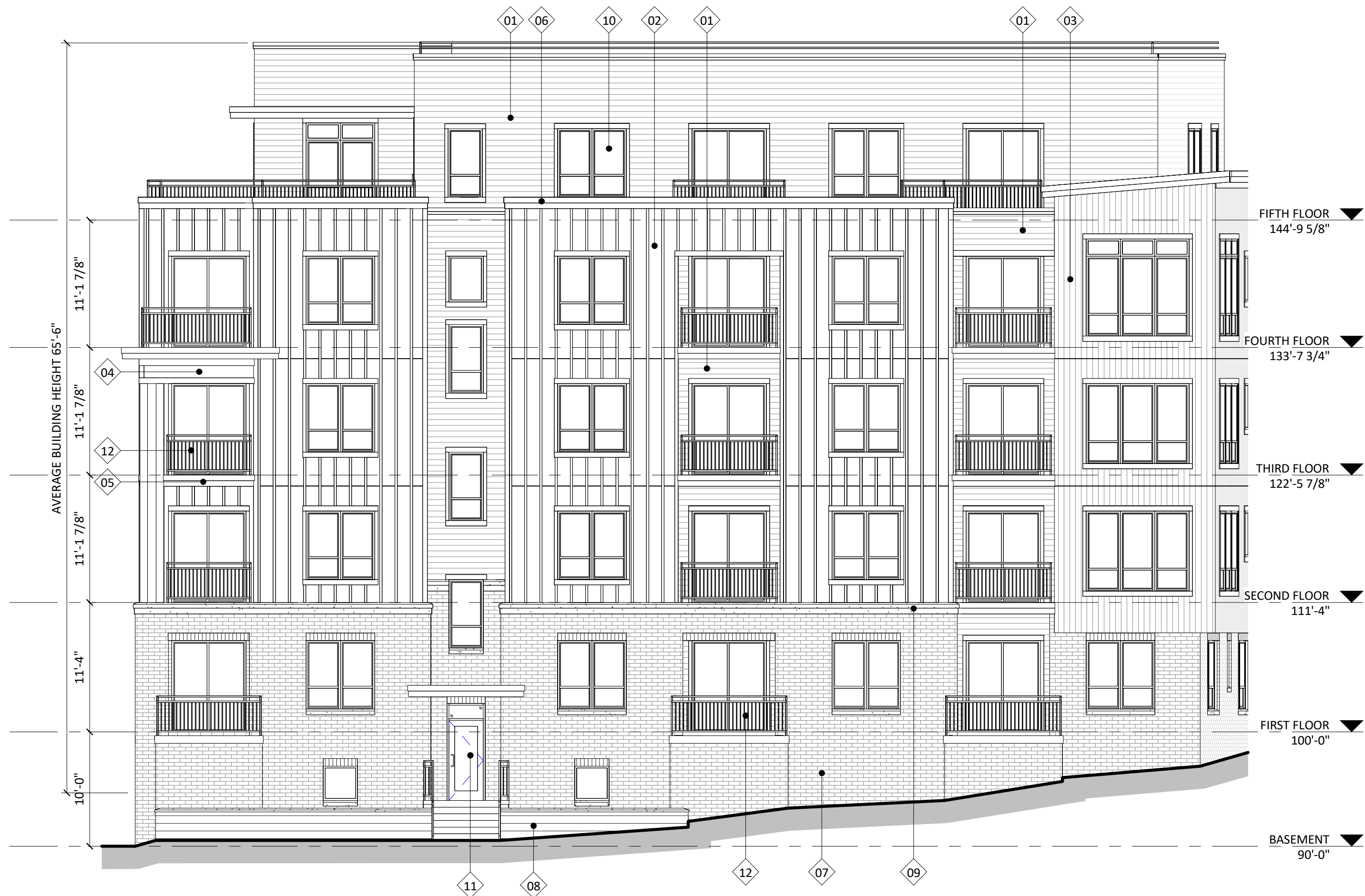
2 WEST ELEVATION ALONG N. WHITNEY WAY 1/8" = 1'-0"
