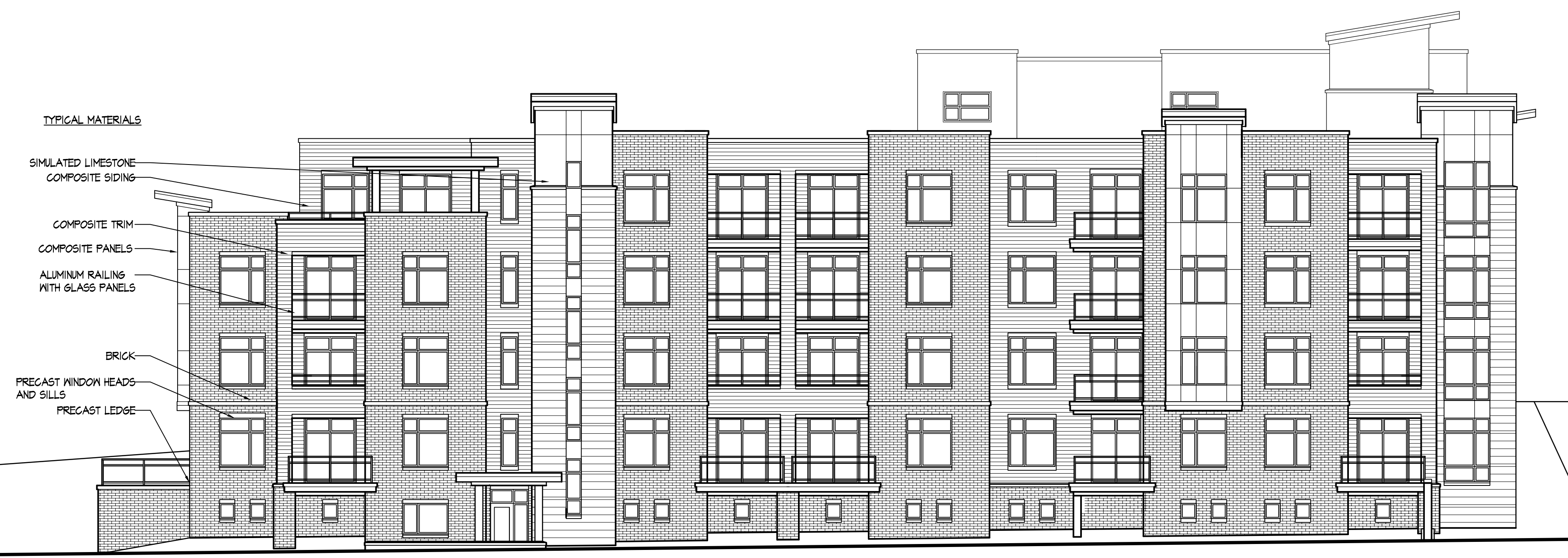
NORTH ELEVATION ALONG UNIVERSITY AVENUE 3/8" = 1'-0"
