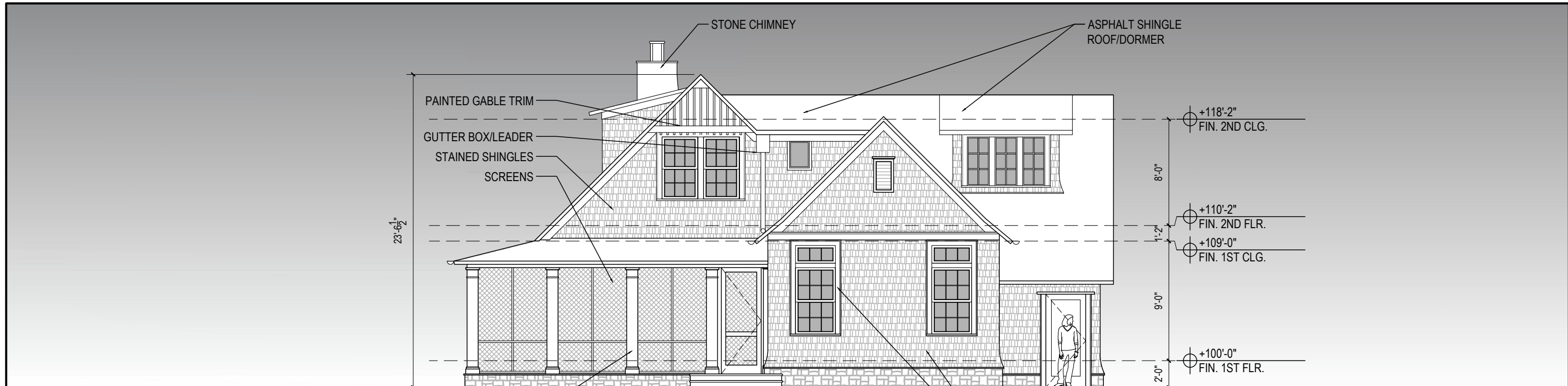
1 SOUTH ELEVATION (BACKYARD) 1/8"=1'-0"
