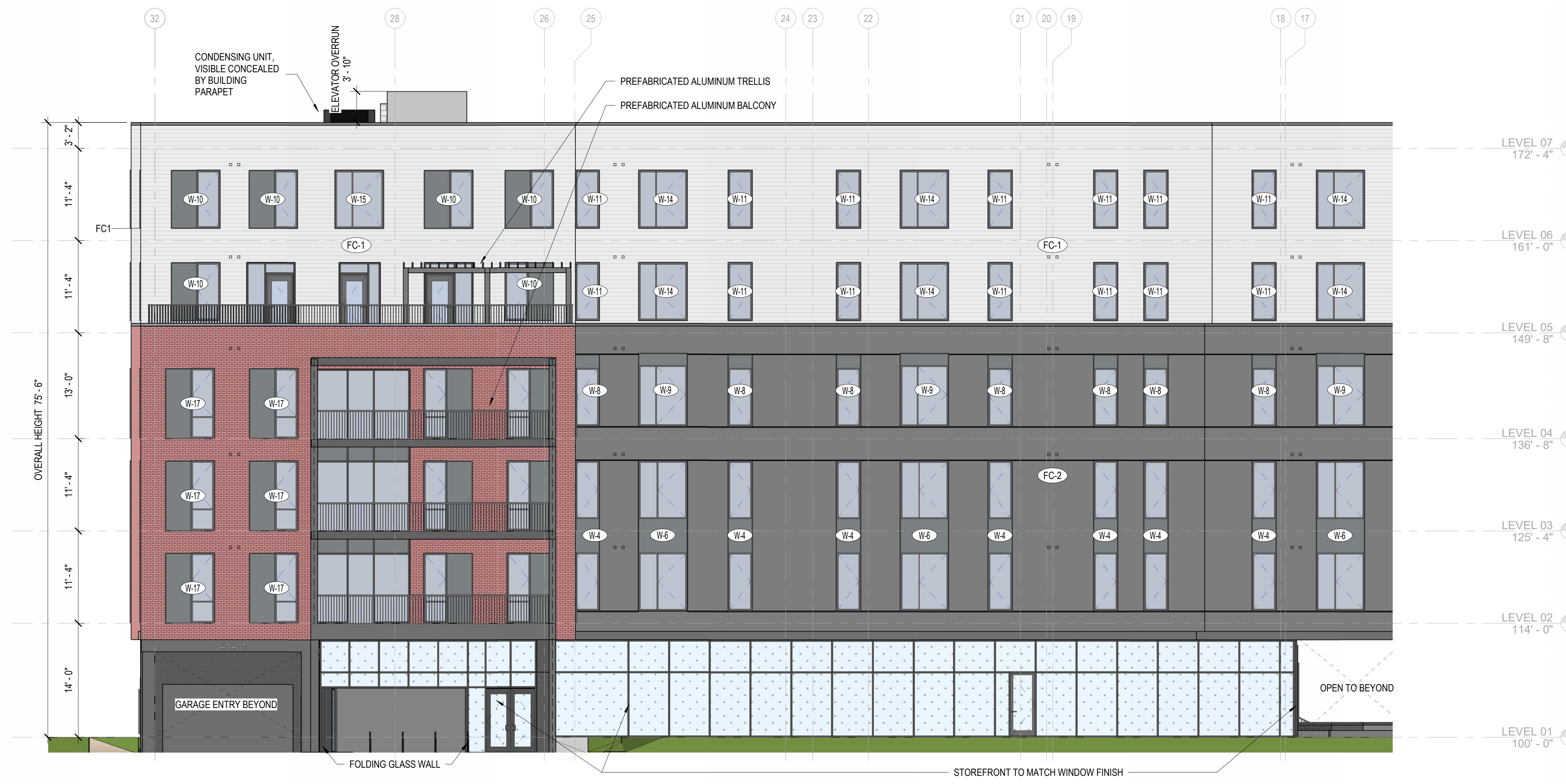
E3 ENLARGED ELEVATION - NORTH - AREA A A6.102 1/8" = 1'-0"
