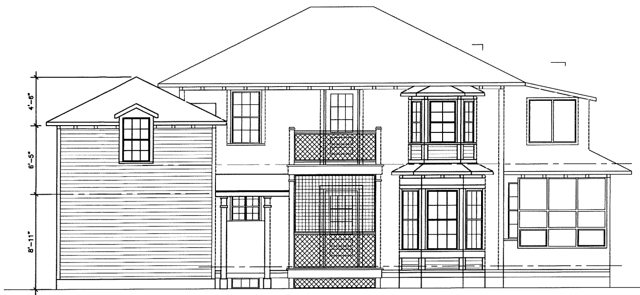
3 WEST EXTERIOR ELEVATION 1/4"=1'-0"
