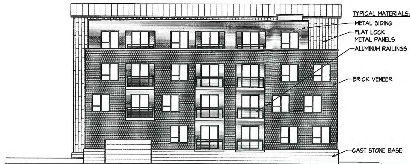
1 North Elevation - Rear View A-2.2 1" = 16'
