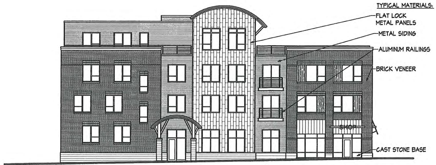
1 West Elevation - Patterson Street A-2.1 1" = 16'
