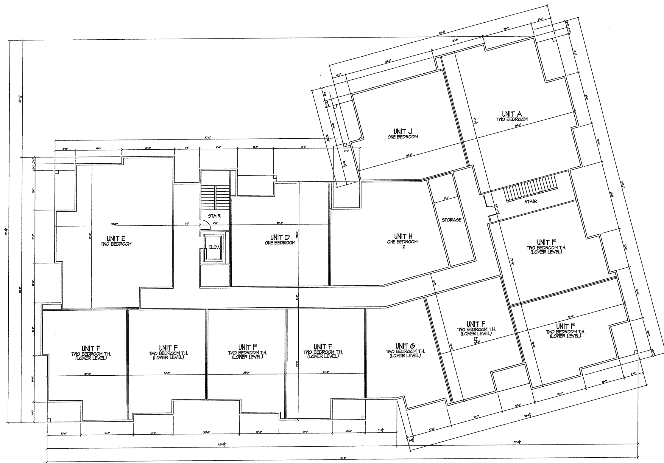
SECOND FLOOR PLAN 1/8" = 1'-0" 2nd FLOOR AREA: 13,386 S.F.
