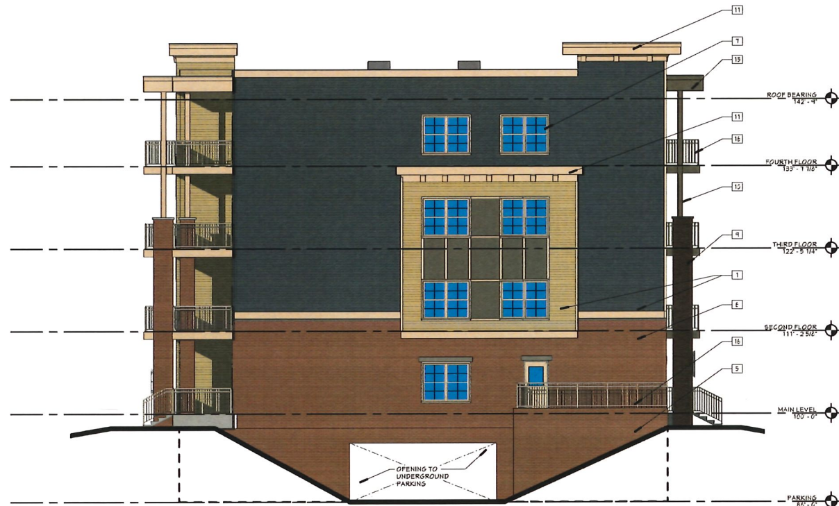
1 A4.4 BUILDING 3 - SOUTH ELEVATION 1/8" = 1'-0"
