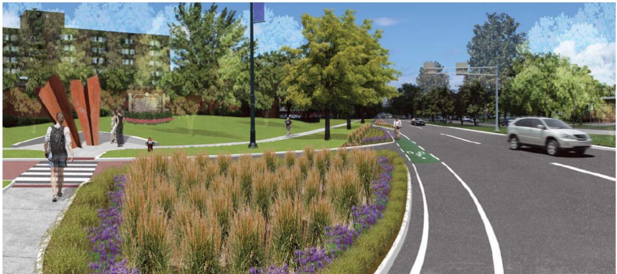
FIGURE 25 View of design option looking northeast along West Washington Avenue from South Park Street toward the capitol building. Bump-outs and landscaping help delineate the bike lanes and provide a safer crossing for pedestrians. Public art could help make this intersection a gateway into the capitol.
